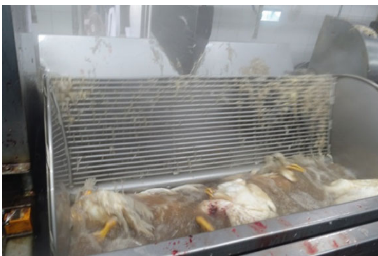
Fig. 11.7 The ducks are immersed into hot water to facilitate easy mechanical plucking
