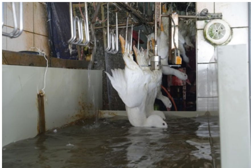
Fig. 11.4 The ducks are stunned by slipping through the electrified water
