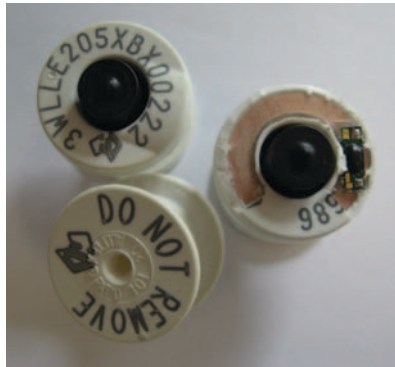
Figure 45. NLIS Breeder devices made by Allflex. The tag on the right with the top cut away shows the coil of copper wire used as an antenna and the small microchip. The microchip is found under the 'bump' on the front of the tag.
