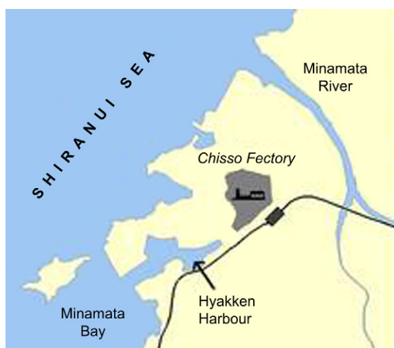
FIGURE 23.3 The Chisso factory, responsible for the methylmercury pollution and its wastewater routes. Instead of discharging its waste into Hyakken Harbour (the source of original contamination), from September 1958 it discharged wastewater directly into Minamata River. The immediate effect was the death of fish at the mouth of the river, and from that point on new Minamata disease victims began to appear in other fishing villages up and down the coast of the Shiranui Sea.
