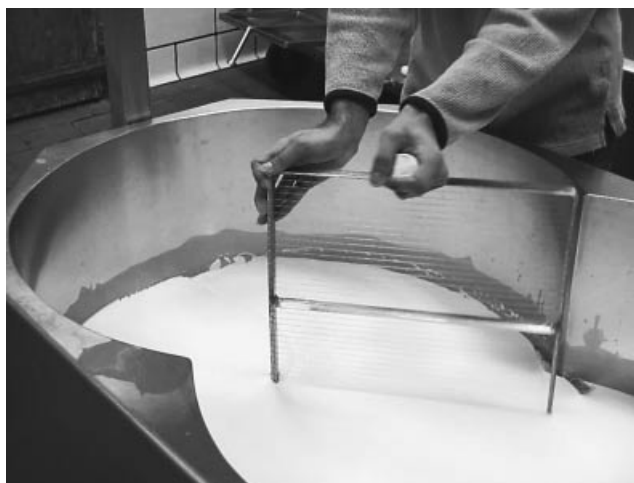
Figure 11.2. Cutting of rennet curd.
