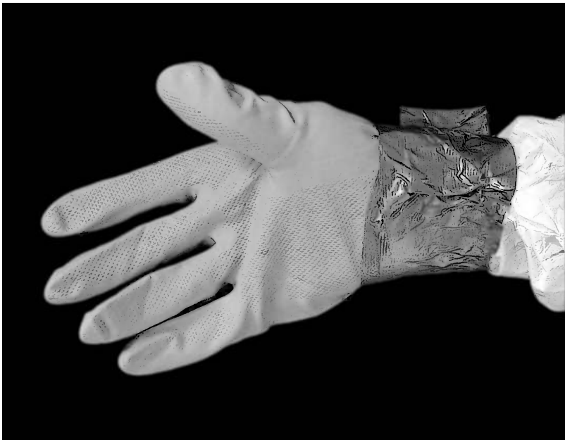
Fig. 2 The Tyvek suit is taped onto the outside of gloves and boots to protect against exposure to hazardous material.
