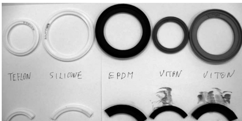
Figure 17.21 New gaskets (top) and after the chemical resistance test (bottom).
