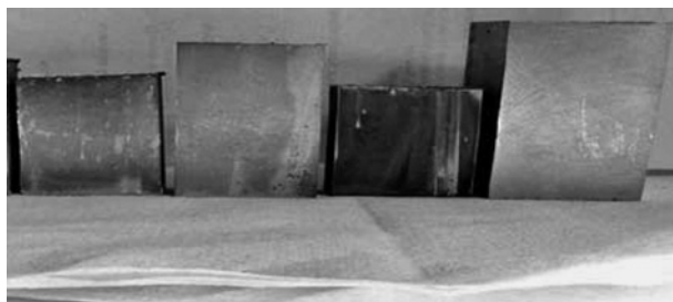
Figure 3.19 Prevention of blackening by ATMP and HEMP. Conditions: 50°C and 72 h soak. Phosphoric acid 2%, + 2 g L -1 HEMP (20 h), + 2 g L -1 HEMP (72 h), + 2 g L -1 ATMP.
