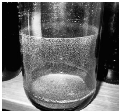
Figure 6.3 Deposit of calcium carbonate crystals from mineral water left in open bottle.
