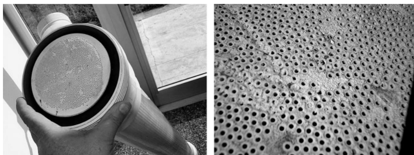
Figure 8.45 Hollow-fiber membrane fouled by an excess of bentonite.
