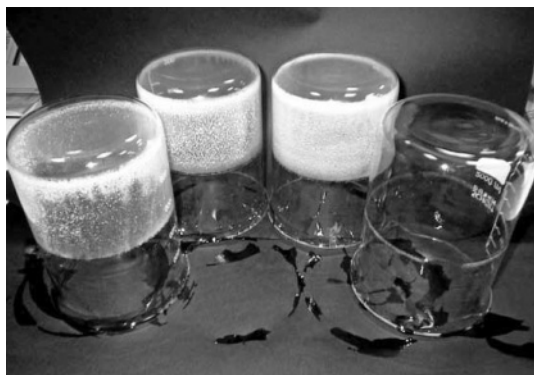
Figure 3.40 The absence of alumina deposit confirms the efficiency of gluconate.
