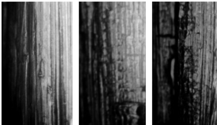
Figure 8.24 Surface modified by ageing (photomicrograph).
