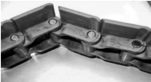
Figure 7.66 Stress cracking of POM chains from acidic cleaning in the field.
