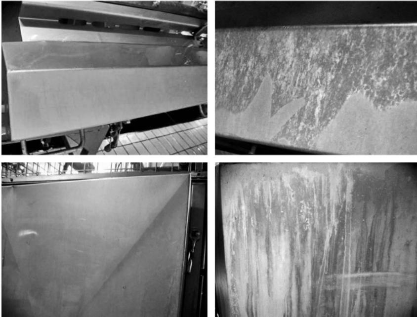
Figure 11.9 Cleaning problem from unsuitable concentration of detergent.
