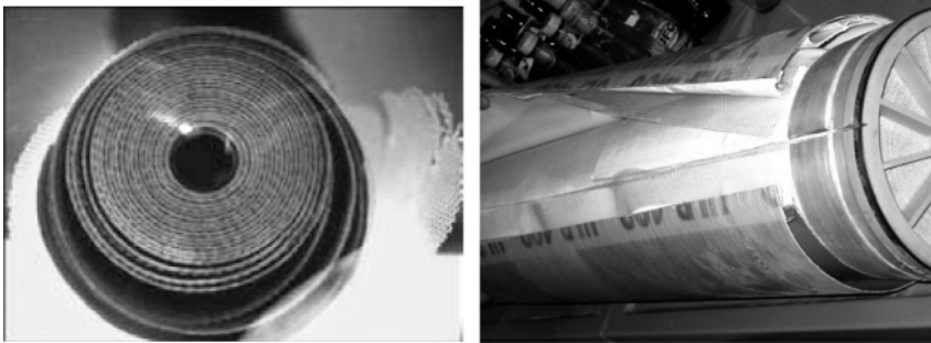
Figure 12.13 Axial path of the SW membrane.
