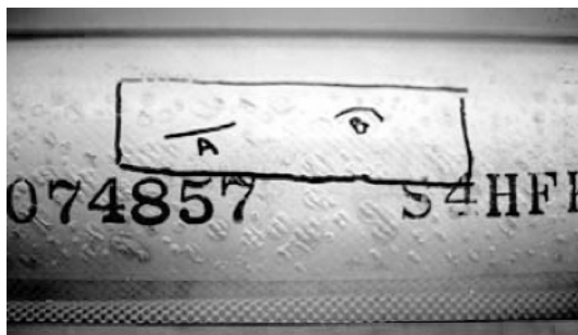
Figure 12.9 UF spiral wound membrane blistered by hot whey feeding.
