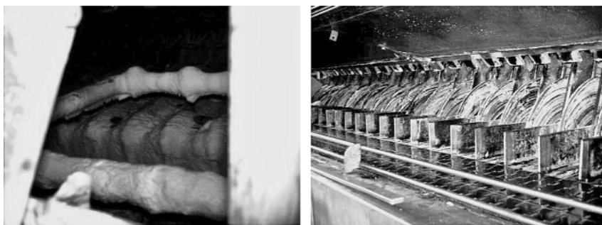
Figure 6.40 Limestone in rinse section and discharge (mineral water bottling).
