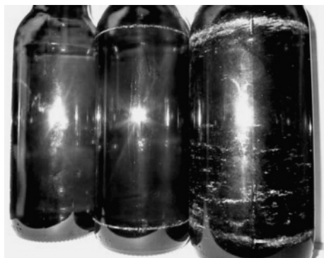
Figure 6.36 Scuffing in the life of a bottle.
