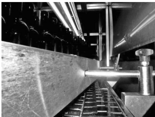
Figure 7.47 UV-lamps microbiologically protect the environment around a conveyor running in stainless steel reflecting tunnel.
