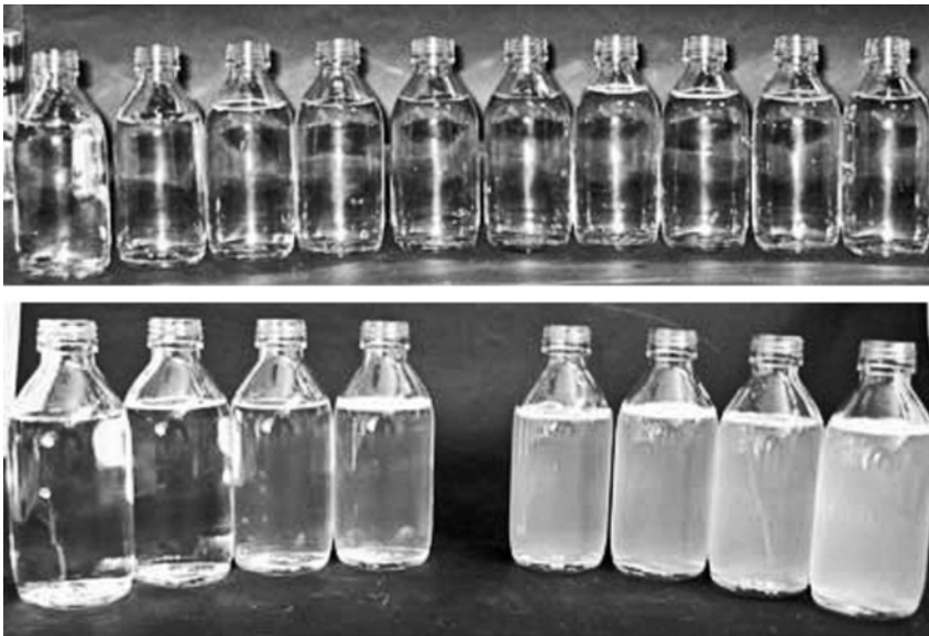
Figure 7.44 Test of FAEC efficacy in preventing turbidity.
