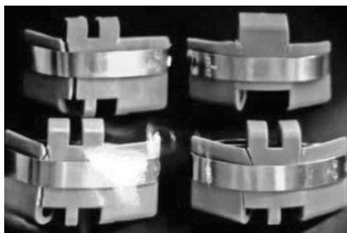
Figure 7.64 Stress cracking on POM chains exposed to acids.
