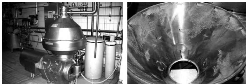
Figure 8.20 Separator and example of incomplete cleaning.
