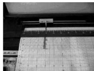
Figure 7.9 (a) Tracks running regularly. (b) Poor lubricity makes the same tracks jump.
