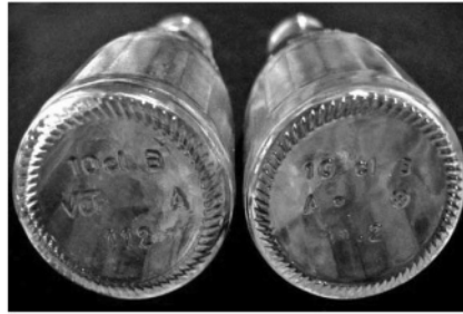
Figure 7.16 Different micro-friction from different shape of the bottle bottom.
