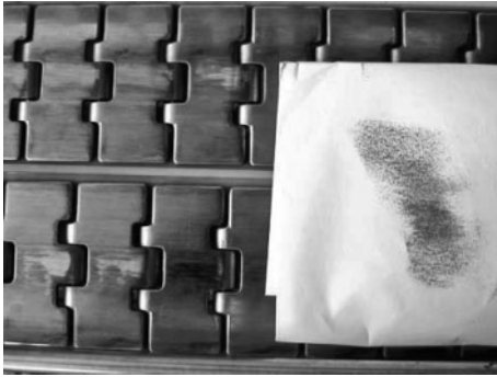
Figure 7.8 Oily deposit containing black oxides.
