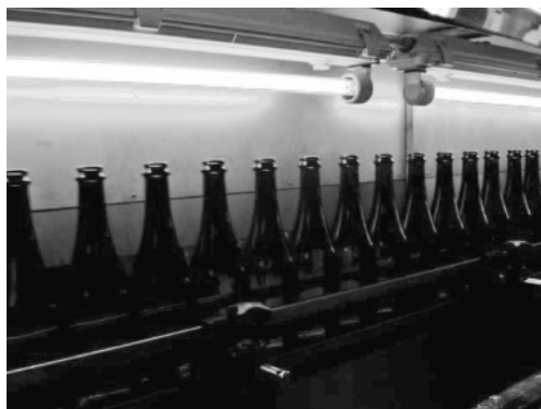
Figure 15.6 Example of conveyor protected by UV lamps before filler. UV rays are reflected inside a stainless steel tunnel which covers the track.
