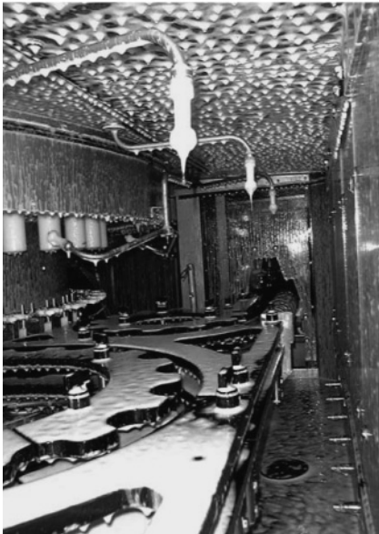
Figure 6.52 (a) EFC foam CIP and (b) bottle sterilization with PAA (courtesy of JohnsonDiversey).
