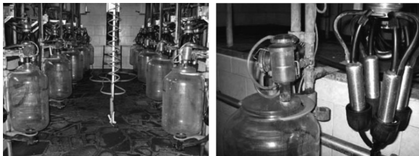
Figure 13.9 Jars and their valves showing milkstone formation due to unsuitable cleaning.
