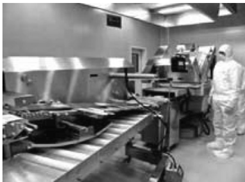
Figure 15.4 ISO 5 (class 100) clean room (courtesy of Sinteco).
