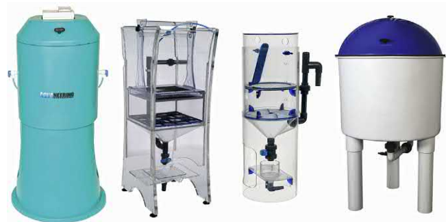
FIGURE 26.5 Mass Embryo Production Systems (MEPS). Large numbers of broodstock fish can be housed and spawned directly inside these devices, facilitating on-demand collection of synchronized embryos. From left to right, an example of a polyethylene MEPS, large (60 L, 200 fish) and small (13 L, 40 fish) acrylic MEPS, and a fiberglass-reinforced polyester MEPS. Courtesy of Aquaneering Inc., Courtesy of Tecniplast Aquatic Solutions and Courtesy of Pentair Aquatic Eco-systems.
