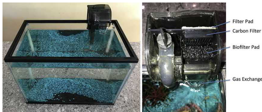
FIGURE 26.8 Hang-on Filter. With the application of a hang-on filter to an otherwise static holding tank, the useable lifespan of the culture water can be significantly extended. A small powerhead pump draws water up and out of the tank. The water then passes through a basic mechanical filter pad, activated carbon filter, and biological filter sponge before freefalling back into the holding tank, offering an opportunity for gas exchange.
