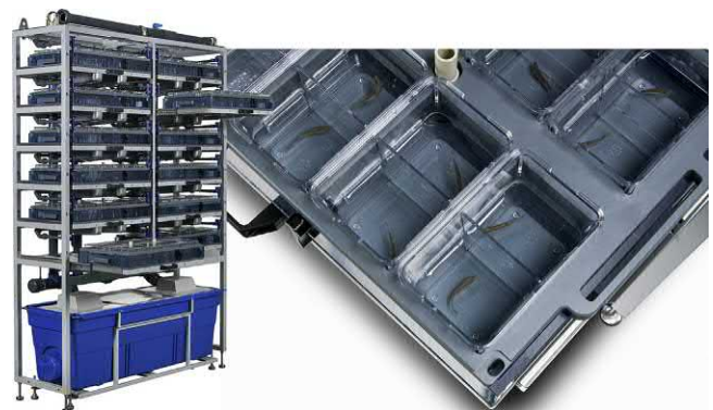
FIGURE 26.13 Genotyping Rack with under-rack sump. Photo courtesy of Tecniplast Aquatic Solutions.
