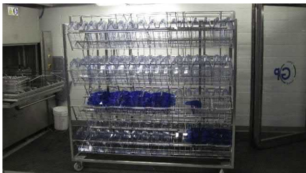
FIGURE 27.11 Image of Tecniplast cage wash presentation rack loaded with fish tanks and components, prepared for entry to Tecniplast Cage and Rack Washer. Photograph courtesy of IWT/Tecniplast.
