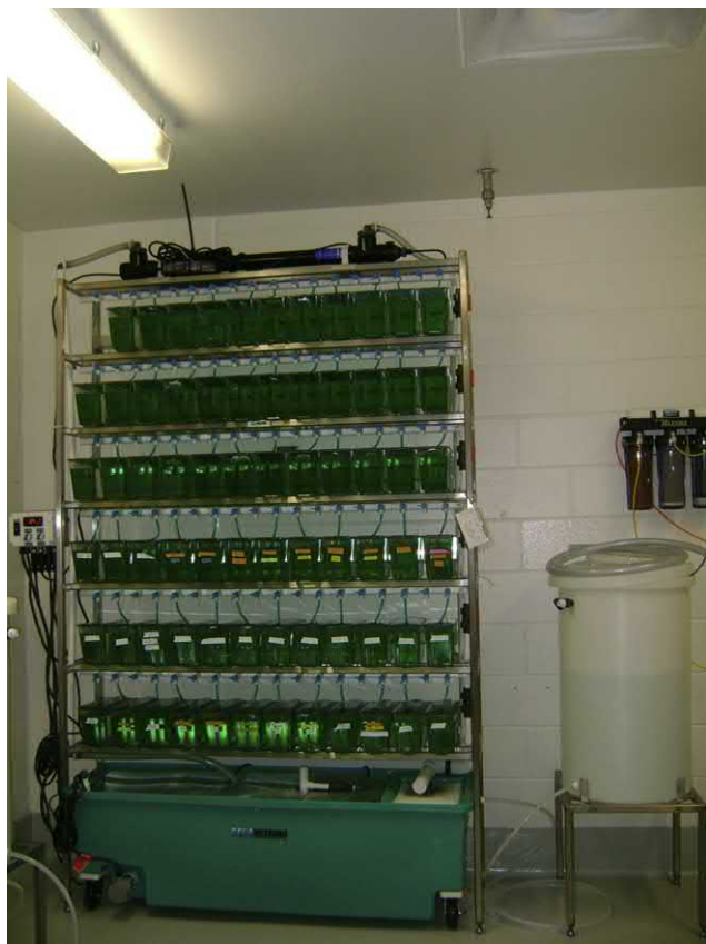
FIGURE 36.9 Example of a self-contained single rack, which could be used for quarantine. Compact racks are also available that can be placed in small areas, such as an isolation cubicle or on a benchtop.
