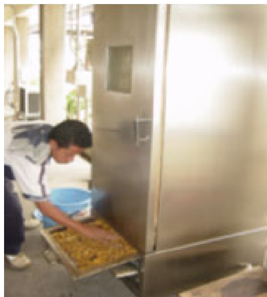
Fig. 37: Small-scale smokehouse (sawdust is placed on the smouldering tray)
