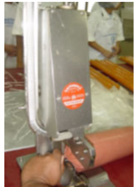
Fig. 35: Manually operated sausage clipping machine with clip rails (left)
