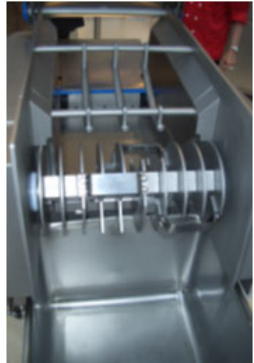
Fig. 57: Frozen meat cutter with rotating round knives for cutting out pieces/chips from frozen meat blocks
