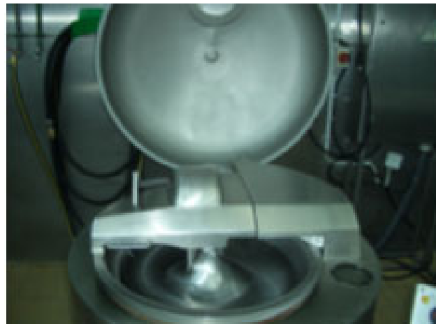
Fig. 30: Vacuum cutter; lid can be hermetically closed for vacuum treatment of batter in the bowl
