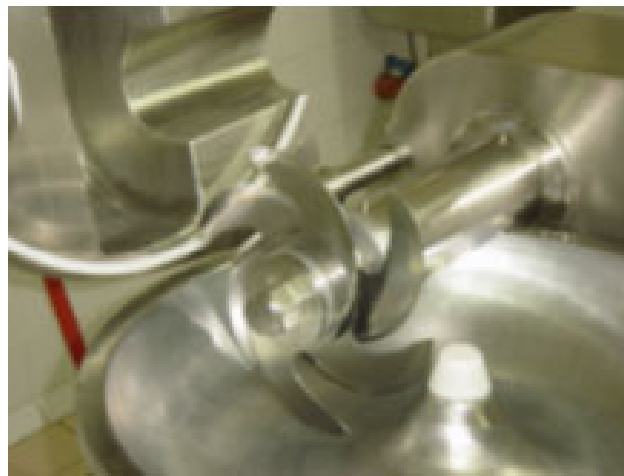
Fig. 26: Bowl cutter assembled with 6 knives
