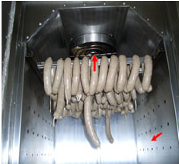
Fig. 41: Small smokehouse, inside view, air/smoke circulation forced by extraction fan on top (arrow) and re-circulated through openings in double jacket side wall (arrow)
