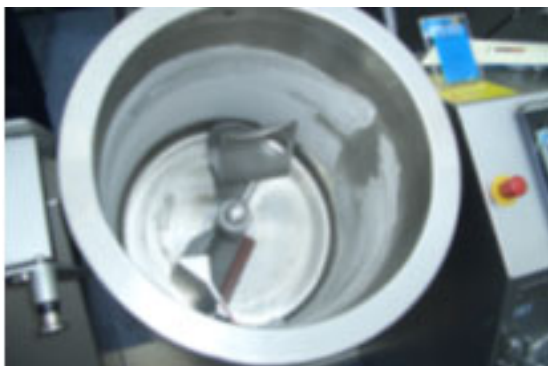
Fig. 48: Tumbler with double jacket for refrigeration and vacuum pump/motor device
