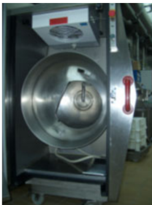
Fig. 49: Tumbler inside mobile refrigerated housing
