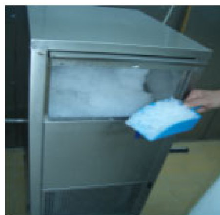
Fig. 56: Ice flaker with storage compartment
