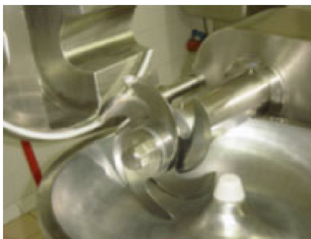
Fig. 26: Bowl cutter assembled with 6 knives
