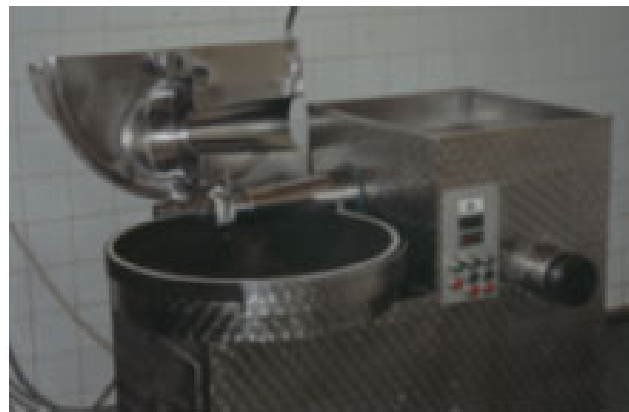
Fig. 29: Bowl cutter–grinder combination (twin model) with bowl cutter (60 litres capacity) and meat grinder (114 mm orifice diameter)
