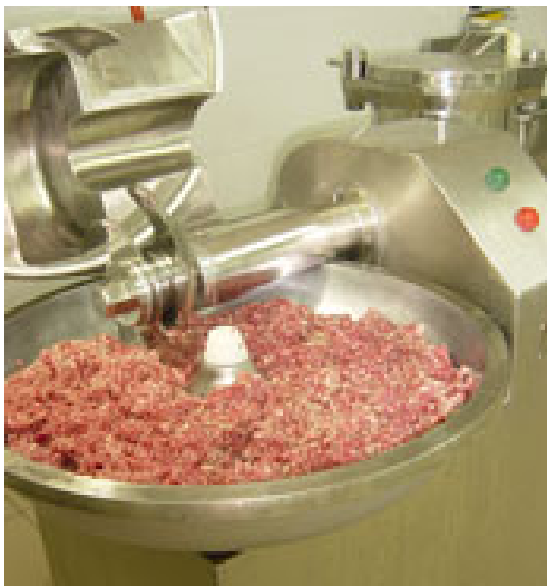
Fig. 28: Bowl cutter filled with meat for chopping
