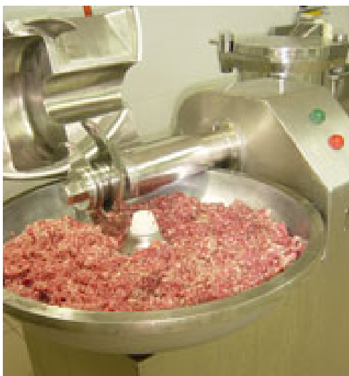
Fig. 28: Bowl cutter filled with meat for chopping
