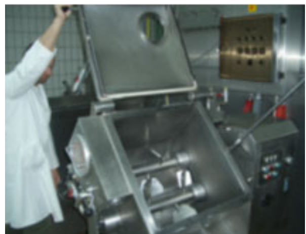
Fig. 52: Blender with lid for hermetic closure for vacuum treatment; can be declined for emptying
