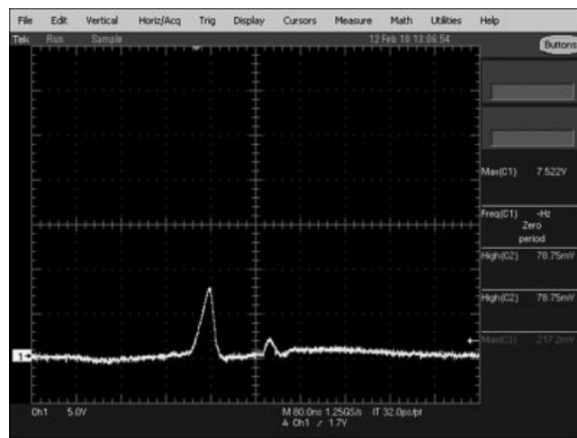
Figure 37.4 Typical short-duration pulse (nanoseconds) as a function of time, as shown on a conventional oscilloscope measurement device. At high voltages, short-time reflections may accompany the pulse. In the picture, each vertical division represents 80 ns and each horizontal division represents 2500 V.
