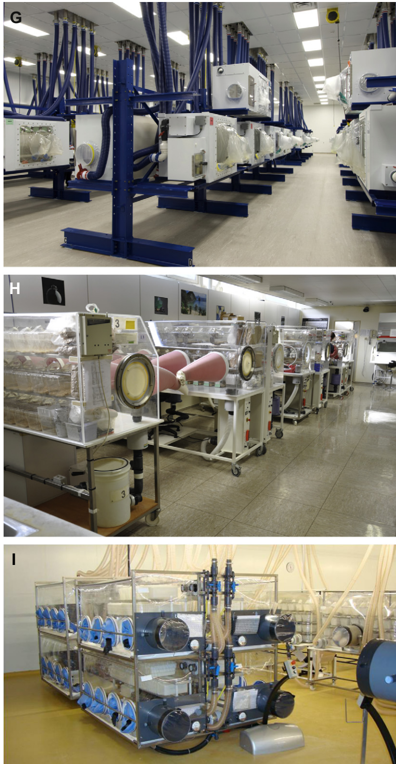
Figure 4.6.2—Cont'd. G. Rigid-body, positive-pressure standard fixed isolators, on two levels, for small breeding projects, with standard connection port (photo credit: Taconic). H. Rigid-body, positive-pressure standard movable isolators, for breeding projects, with rapid-transfer door (photo credit: Institut Pasteur Lille). I. Flexible-film, positive-pressure, standard movable isolators, on two levels, for small breeding projects, with standard connection port (photo credit: Janvier).
