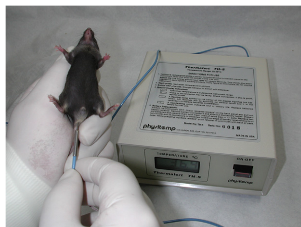
Figure 5.1.17 Fixation of a C57BL/6 mouse during temperature recording. Note: this is an adult animal.
