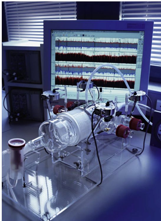
Figure 2.7.4 Schematic drawing of the head-out body plethysmograph and photograph of a complete system (Fraunhofer ITEM, Hannover, Germany). The figure illustrates the exposure system and the equipment used for the measurement of tidal mid-expiratory flow ( EF_{50} ), tidal volume (VT), expiratory time (TE), inspiratory time (TI) and breathing frequency (f). The conscious animal was placed in a glass plethysmograph that was attached to a head exposure chamber (see photograph: chamber with graph plethysmographs). The output of a jet nebulizer was directed to the inlet of the head exposure chamber that was continuously ventilated with a bias flow of 0.2 l/min. Before data collection, mice were allowed to acclimatize for 15 min in the body plethysmograph. Schematic drawing adapted from Glaab et al., 2001.
