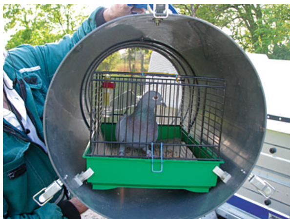
Photo 5.57 Pigeon-baited mosquito trap (O. Šebesta)
