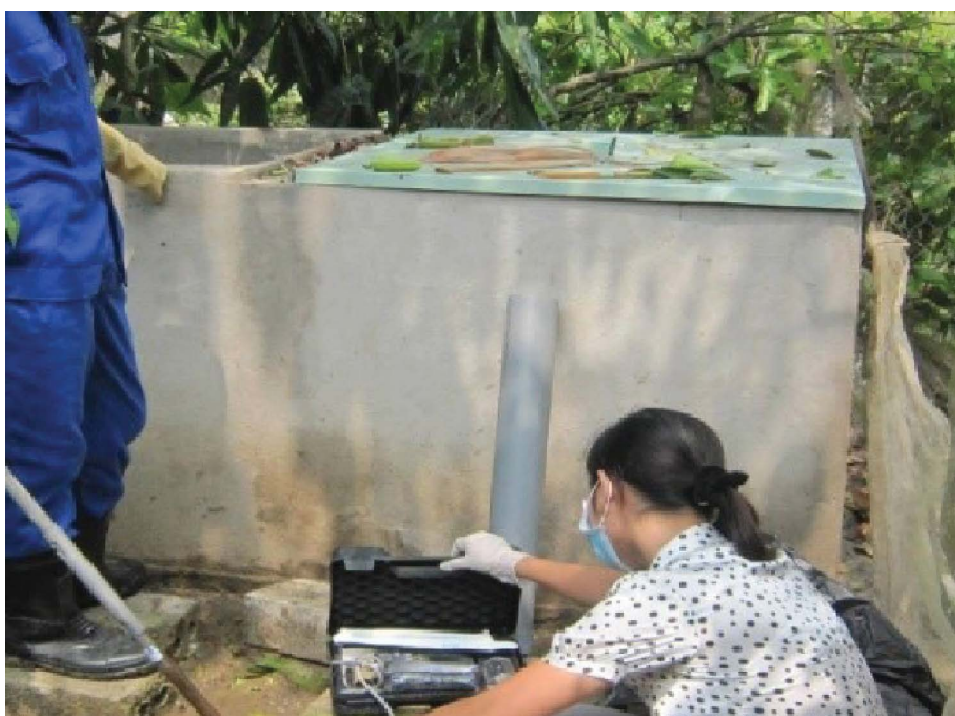
Fig. 13.4. The experimental field model used for combined human and animal waste composting.
