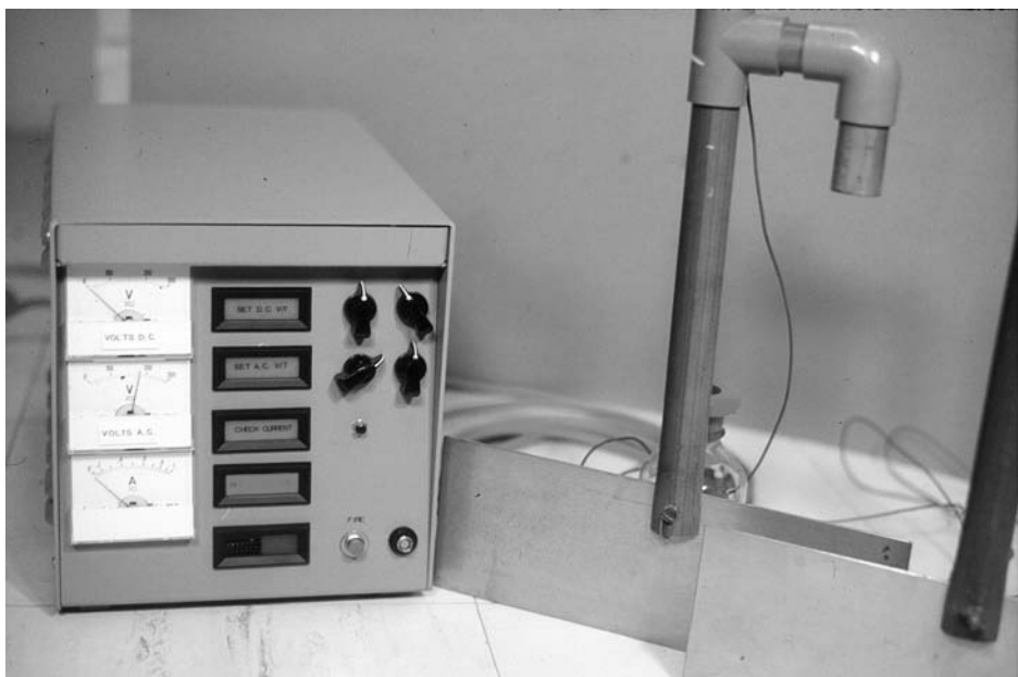
Figure 11.5 The electroanaesthesia control unit and stainless steel plate electrodes used in the author's laboratory. Note the voltage and time selector switches at top right, the indicator panels which light in sequence to guide the user through the firing procedure and the stainless steel plate electrodes used in tanks.
