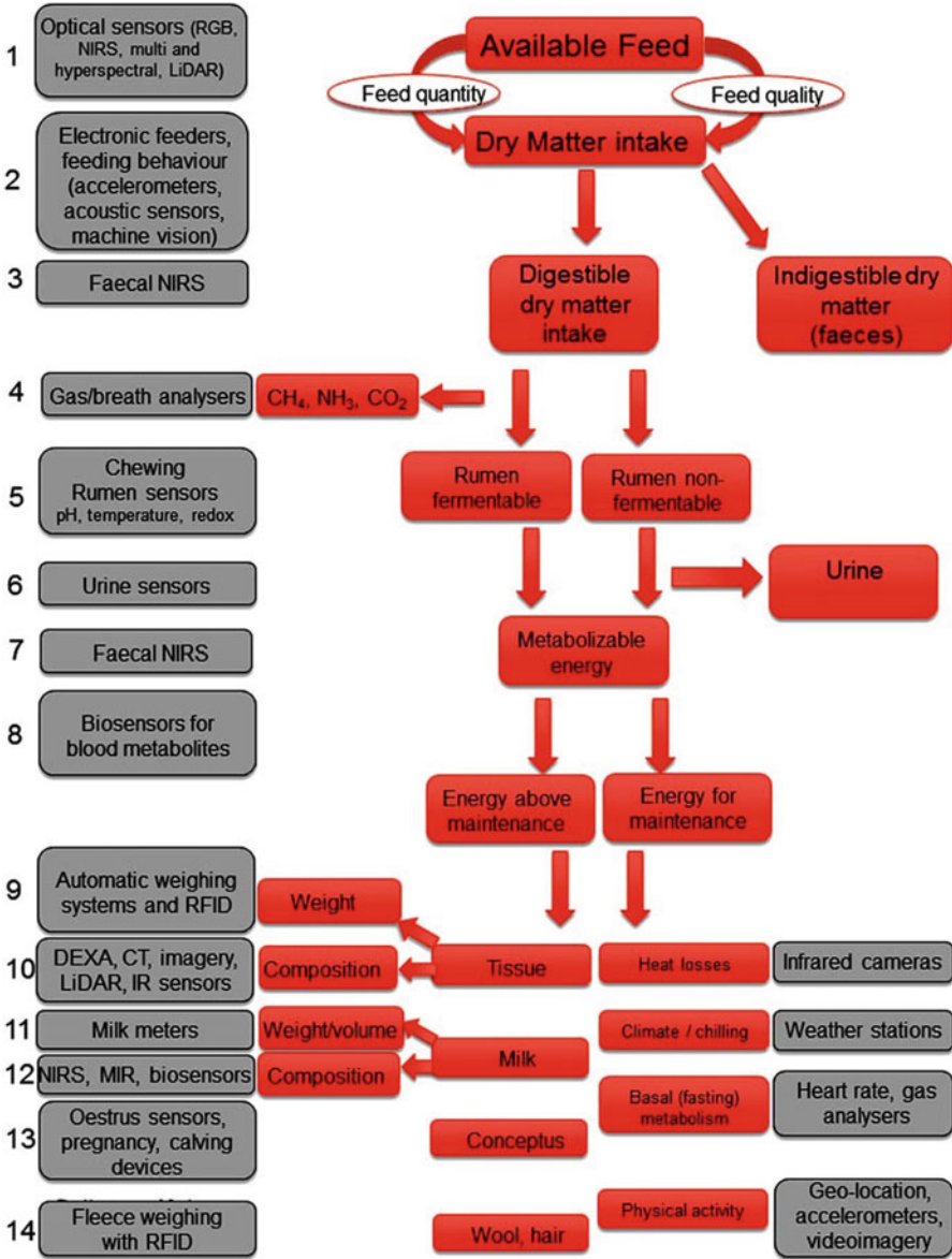
Fig. 11.4 A schematic of nutrient flows in dairy systems and the available technologies to measure key nutritional processes. (Reproduced with permission from Gonzalez et al., 2018)
