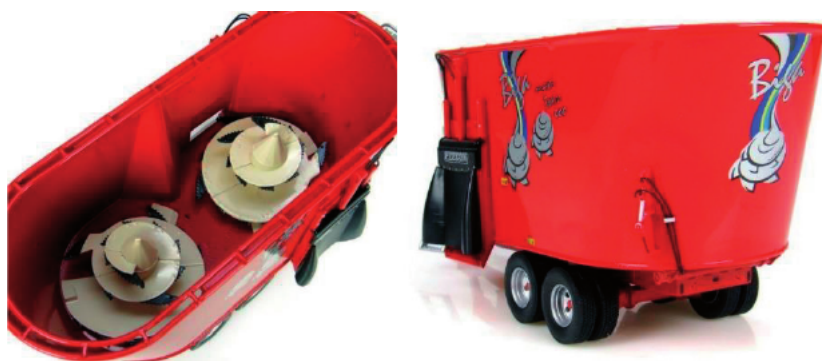
Figure 7. Small format “unifeed” mixer truck, adapted to Lidia cattle (BIGA).
