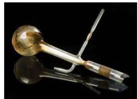
Figure 1.4 A Chamberland filter. Charles Chamberland (1851–1908) discovered that warm porcelain can retain fine particles in solution and, along with Louis Pasteur, showed that bacteria can be filtered out of a solution using a porcelain filter in a glass tube such as the one depicted here. Viruses were first understood as microbes so tiny that they could pass through a Chamberland filter. (Courtesy of Wellcome Library, London. Published under CC BY 4.0.)
