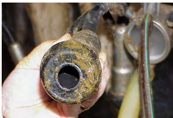
Figure 1. A milking machine liner in use.
