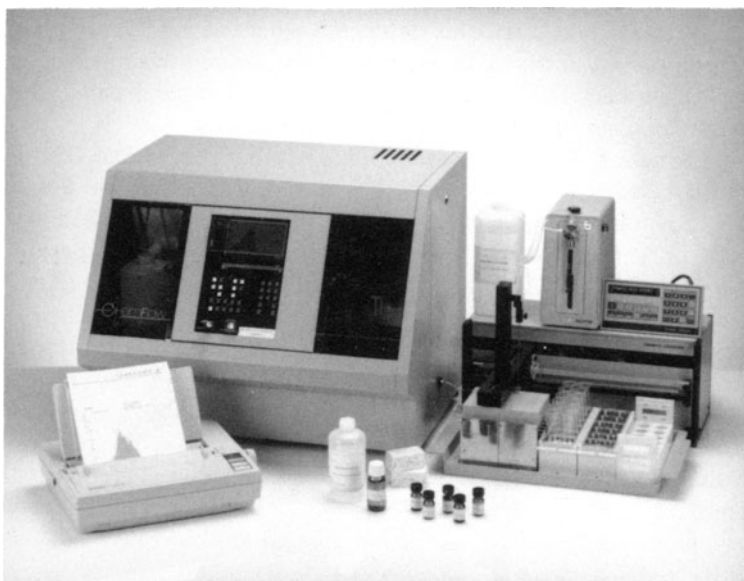
Fig. 9. The ChemFlow system of reagents, automatic sample injector and flow cytometer. (Reproduced by courtesy of Chemunex SA, France.)
