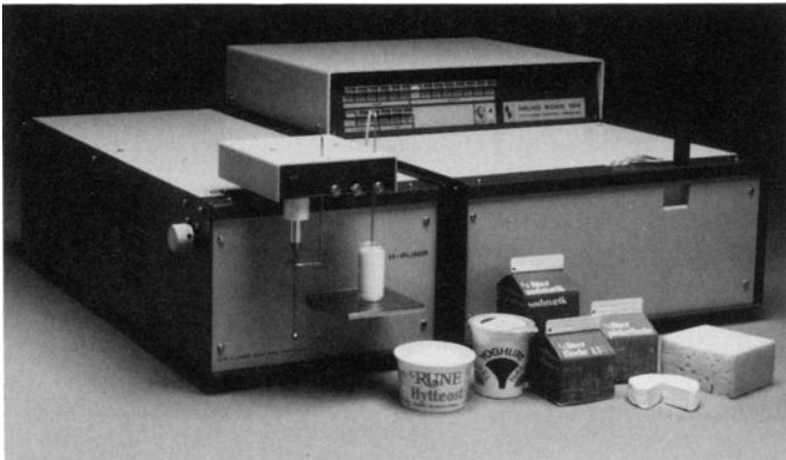
Fig. 12. 1983 version of IR instrument (Milko-Scan 100) for three- or four-component analysis. Measures 90 samples per hour (fat, protein, lactose), manually presented to instrument. (Courtesy of A/S N. Foss Electric, Denmark.)
