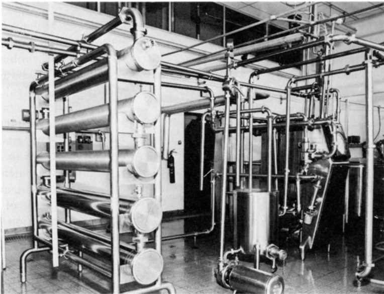
Fig. 8. A heating unit for yoghurt milk, including a balance tank (centre), a plate heat exchanger and a 'zig-zag' holding tube (foreground) that provides a residence time of 8 min. (Reproduced by courtesy of the Northern Ireland Milk Marketing Board.)
