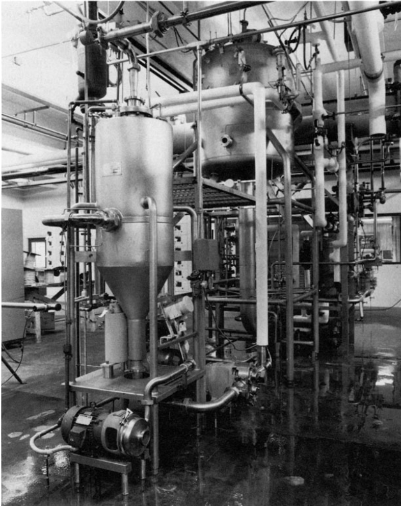
Fig. 3. Ice cream mix UHT pasteurising/sterilising system of the direct steam infusion heating type. The upright vessel in the left foreground is a jacketed steam infusion heater. The vessel in the centre is the steam flash (removal) chamber. The plate regenerator and homogeniser are beyond these two vessels. (Reproduced by courtesy of APV Crepaco, Inc.)
