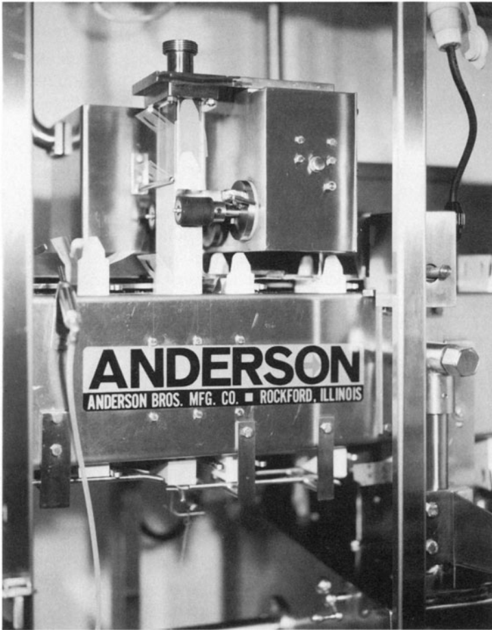
Fig. 7. Carton set-up and filling machine. The machine shown here is for 1-litre home-pack cartons used primarily in the UK. (Reproduced by courtesy of APV Anderson, Inc.)
