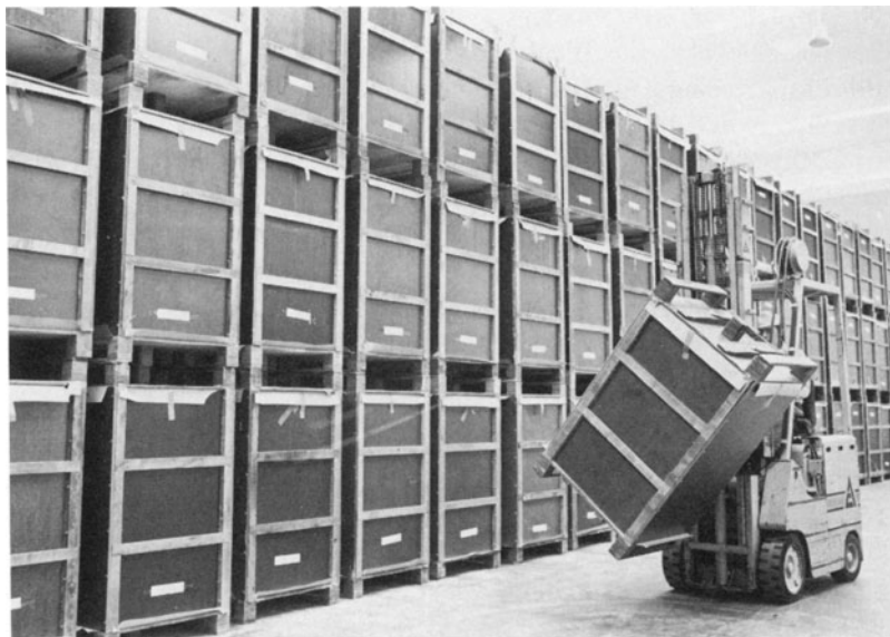
Fig. 31. Mechanical handling for turning large 'block'-shaped Emmental during the maturation period. (Reproduced by courtesy of Tebel-MKT BV, Jarvenpaa, Finland.)
