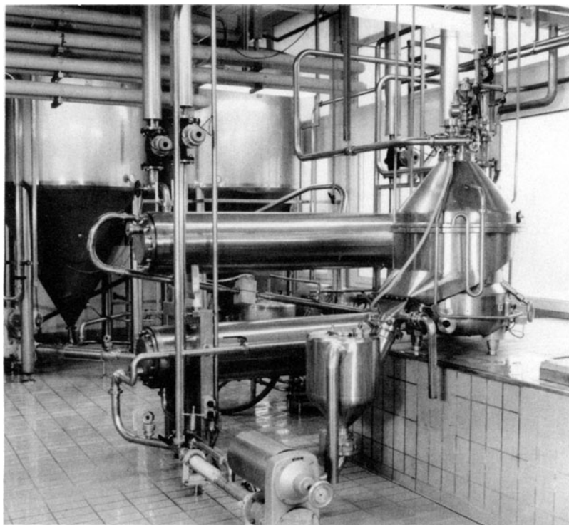
Fig. 10. Thermo-soft cheese line with KDA 30 separator and two tubular coolers. (Reproduced by courtesy of Westfalia Separator, UK.)
