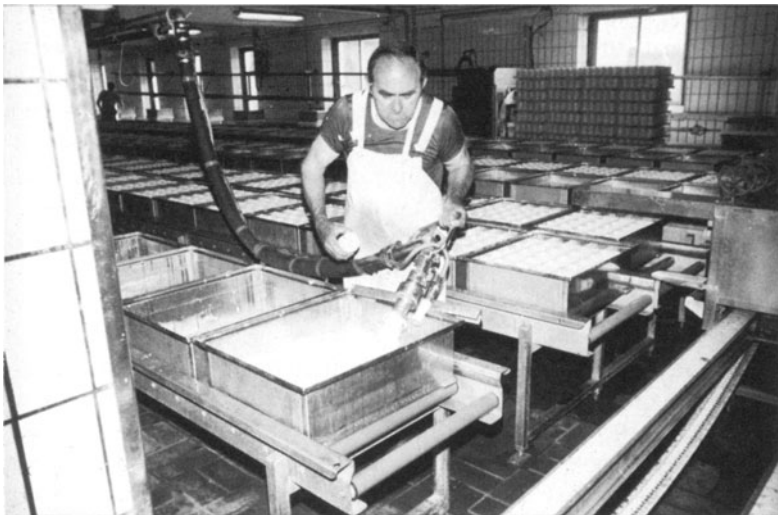
Fig. 14. Cartier system for the manufacture of soft, mould-ripened cheese using small bassines or vats (30 litre). (Reproduced by courtesy of Pierre Guerin.)
