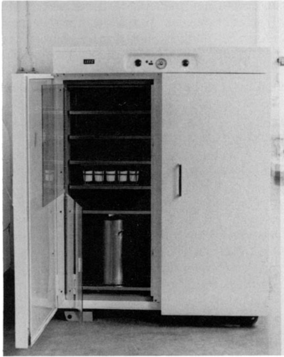
Fig. 9. An electrically operated cabinet that can be used for the incubation of fermented milks on a small scale. These units can be provided also with a refrigeration unit to allow subsequent cooling of the product.
