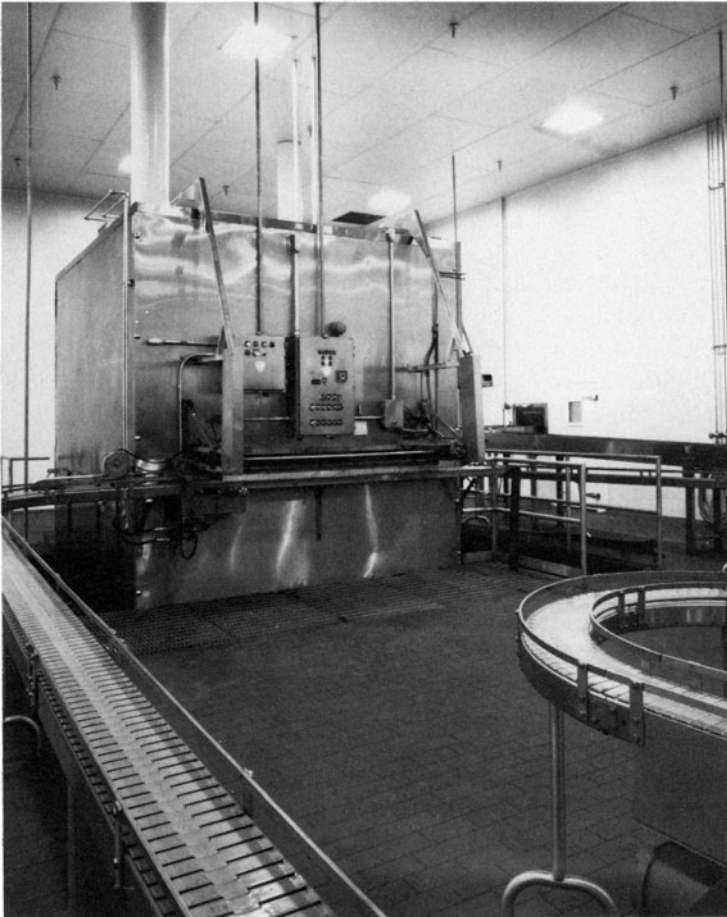
Fig. 8. Contact plate hardener. This type of hardener is the most efficient of hardening systems for ice cream in rectangular cartons. It will accommodate round containers which have large area flat tops and bottoms, but efficiency is reduced because package configuration on the plate prevents contact with as much container surface as in the case of rectangular cartons which fully fill the plate area. (Reproduced by courtesy of APV Crepaco, Inc.).
