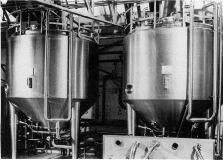
Fig. 7. These multi-purpose tanks can be employed for heat-treating the process mix, the incubation stage and, finally, cooling the finished product. (Reproduced by courtesy of Goavec SA, Alencon Cedex, France.)
