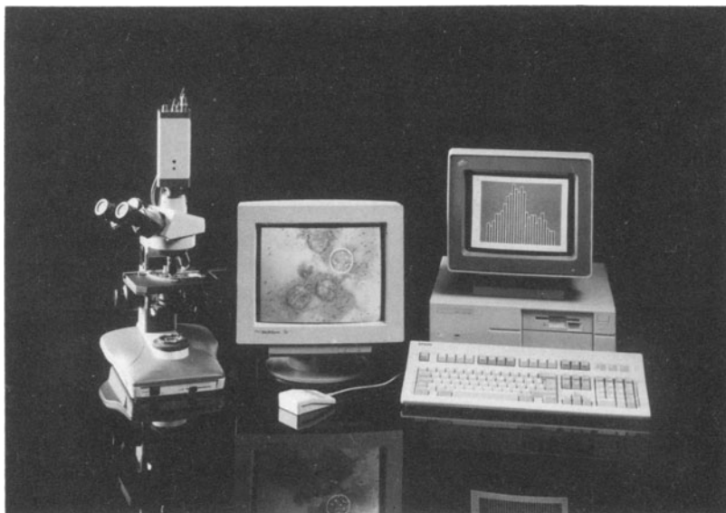
Fig. 5. Image analyser for the semi-automated counting of bacteria on DEFT slides. (Reproduced by courtesy of Perceptive Instruments, Halstead, UK.)
