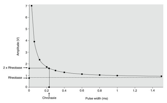
**Figure 14.1** A strength-duration curve from a temporary atrial lead in a horse displays the combinations of pulse strength and duration above which consistent capture is achieved. The rheobase is the lowest voltage at (infinitely) long pulse duration that results in capture. The chronaxie is the threshold pulse width at twice rheobase.
