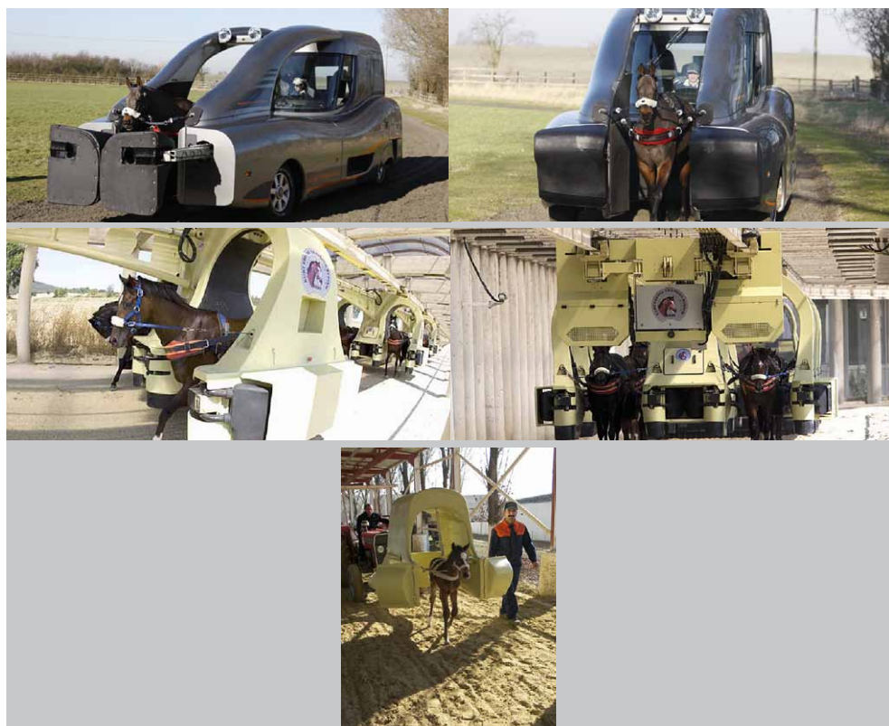
Figure 4. Kurt Systems' horse training vehicle and track system for training horses without riders.
