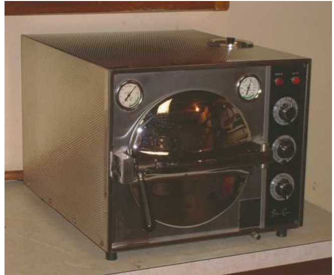
FIGURE 19-2 An autoclave provides high-pressure steam heat to sterilize surgical instruments.
