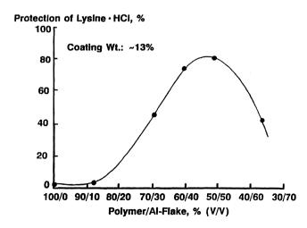
Fig. 12. Effect of the ratio of polymer:pigment volume on the ruminal protection efficiency of a rumen-stable coating applied to lysine-HCl pellets (coating weight  $\sim$ 13%). Al-flake was treated with stearic acid.
