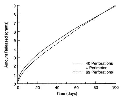
Fig. 12. Comparison of the predicted amount released versus time for the Paratect<sup>®</sup> flex diffuser made with coated and uncoated edges.<sup>8</sup>
