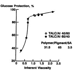
Fig. 13. Effect of polymer molecular weight (or inherent viscosity) on coating efficiency of a rumen stable coating applied to glucose.
