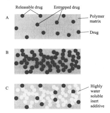
Fig. 7. Effect of loading (or addition of inert, highly water soluble additive) upon the formation of pores in an inert matrix. At low drug loading drug must release via diffusion through the matrix (A). At higher drug loading (B), or if an inert, highly water soluble additive is included in the formulation (C), then following the dissolution of the drug or inert additive after the gradual imbibement of water and formation of fluid filled pores, drug can become released via these pores.
