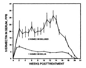
Fig. 6. Concentration of ivermectin in serum of cattle treated either with one or two IVOMEC<sup>®</sup> SR boluses. Cattle were held on pasture in South Texas.
