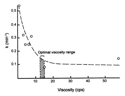
Fig. 1. Drainage rate of various polyvinyl alcohol solutions as a function of solution viscosity (adapted from Ref. 138).
