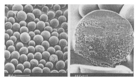
Fig. 1. Biodegradable poly (DL-lactide) microspheres containing 100 mg estradiol and 1.25 g progesterone.
