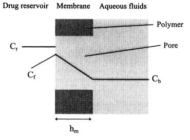
Fig. 3. Physical model describing drug release from porous membrane-type drug delivery systems. The model assumes that boundary layers are insignificant and that fluid within the pores remains unstirred.  $C_r$  is the solubility of drug in the drug reservoir;  $C_f$  is the solubility of drug in the fluids which fill the pores;  $C_b$  is the concentration of drug in the bulk of the fluid phase; and  $h_m$  is the thickness of the rate controlling membrane.
