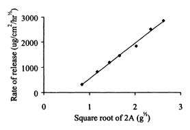
Fig. 5. Effect of initial drug load on the release rate of progesterone from a dispersed matrix system manufactured from silicone (CIDR-B) as a function of the square root of 2A.
