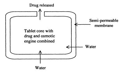
Fig. 2. An osmotic pump for controlled delivery of water-soluble drugs.
