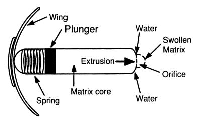
Fig. 6. Winged device of Laby.<sup>7</sup> The wings are held in place by a piece of tape during administration and passage down the esophagus.
