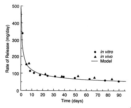
Fig. 14. In vitro/in vivo comparison of release of morantel tartrate from a device with 39 holes.<sup>8</sup>
