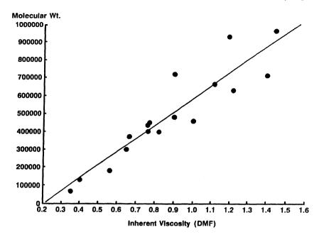
Fig. 8. Relationship between molecular weight and inherent viscosity of poly(2-vinylpyridine-co-styrene 80/20) using DMF as a solvent.
