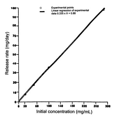
Fig. 21. Drug release rate versus initial drug concentration for the modified Paratect<sup>®</sup> bolus. The slope of the line is 0.34 ml/day and represents the volumetric flux of solution from the device.<sup>78</sup>
