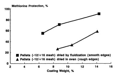
Fig. 17. Effect of rough edges of pellets on protection of methionine. Pellet roughness was altered by drying by fluidization (smooth) or in an oven (rough).
