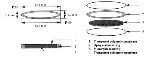
Fig. 7. Schematic representation of the Ocusert<sup>®</sup> system (adapted from Ref. 201).
