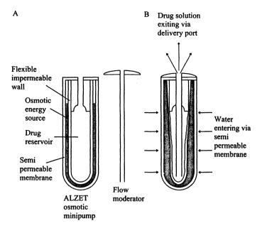
Fig. 8. ALZET osmotic minipump. (A) Major components; (B) osmotic pump in operation.
