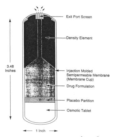
Fig. 16. Cross-sectional view of the IVOMEC<sup>®</sup> SR bolus.<sup>61</sup>
