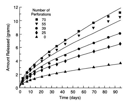
Fig. 13. In vitro and calculated amounts of drug released versus time for devices with 0, 25, 39, 55, and 70 holes.<sup>8</sup>
