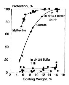
Fig. 9. In vitro ruminal protection and abomasal release of methionine and glucose pellets coated with a rumenstable (reverse-enteric) coating.
