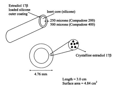
Fig. 6. Compudose 200 and 400 product design. The drug utilization was optimized through knowledge of the mechanism of release (square-root-of time) and determination of the drug depletion zone after insertion. The part of the inner core of the delivery system which does not participate in the release process was replaced by non-drug loaded inert silicone rubber.
