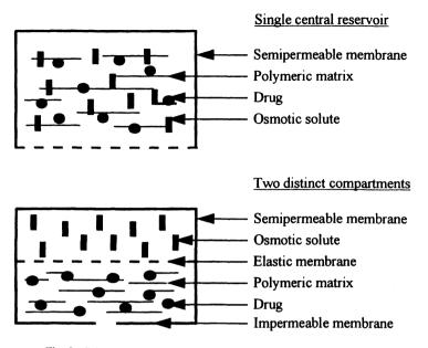
Fig. 8. Schematic representation of the two types of osmotic inserts.
