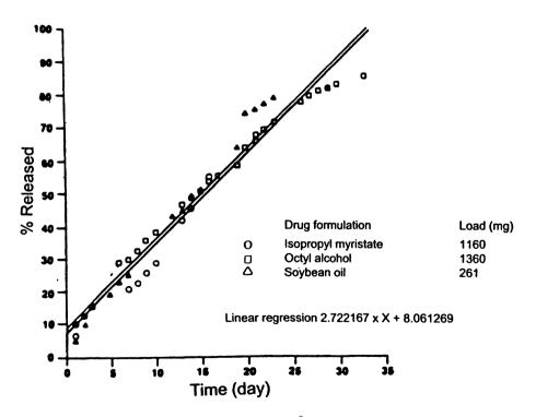
Fig. 22. Percent release versus time for the modified Paratect<sup>®</sup> bolus where various saturated solutions of CP-53,607 in different solvents were evaluated. The data demonstrate that release from this device is independent of the solvent.<sup>78</sup>
