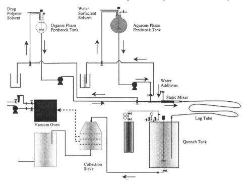
Fig. 2. Diagram of continuous microencapsulation process used to manufacture poly (DL-lactide) microspheres.
