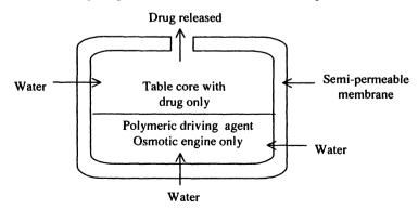
Fig. 3. A push-pull osmotic pump for controlled delivery of insoluble drugs in suspension.
