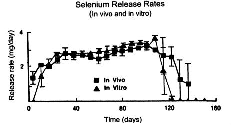
Fig. 19. Rate of release of selenium from push-melt ruminal bolus.
