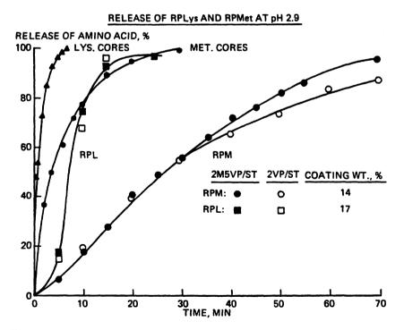
Fig. 10. Release profiles of coated methionine and lysine-HCl pellets incubated in pH 2.9 buffer.
