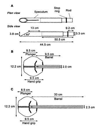
Fig. 2. Schematic diagram and dimensions of some commercially available applicators for the insertion of intravaginal drug delivery systems to farmed animals. A, PRID applicator; B, CIDR-G applicator; C, CIDR-B applicator.
