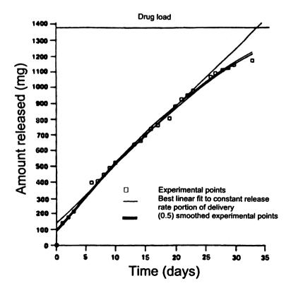
Fig. 20. Release of CP-53,607 from modified Paratect<sup>®</sup> bolus. The device contains 6 g of polyethylene oxide 600 pellets and 28 ml of a 5% solution of CP-53,607 in octyl alcohol. One membrane is sintered polyethylene; the other is impregnated with gelled cellulose triacetate and polyethylene glycol 400.<sup>78</sup>
