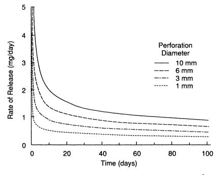
Fig. 11. Effect of hole diameter on the predicted rate of release of morantel tartrate from Paratect<sup>®</sup> flex diffuser assuming the device is 1 mm thick and with one hole.<sup>8</sup>
