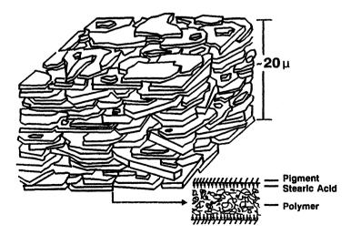
Fig. 14. A brick-and-mortar model for a pH-dependent rumen-stable (reverse enteric) coating.
