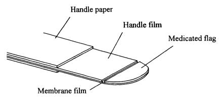
Fig. 6. Schematic representation of the NODS® system (adapted from Ref. 215).
