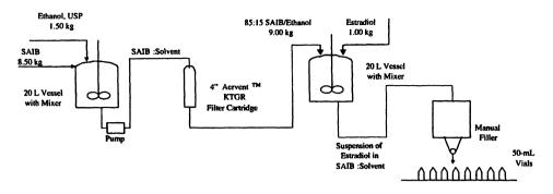
Fig. 5. Process flow diagram for the manufacture of a SABER formulation.
