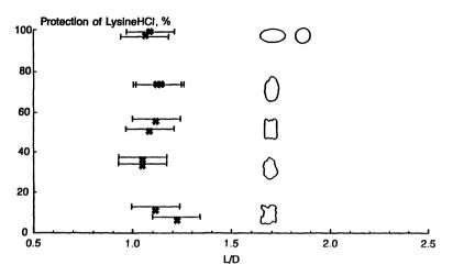
Fig. 19. Effect of pellet geometry on protection of lysine-HCl pellets at 14% coating weight. L/D is ratio of length to diameter (aspect ratio).
