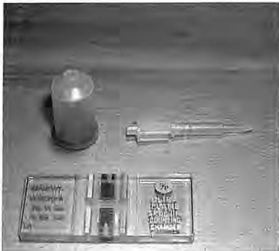
Figure 16-4. White blood cell Unopette system and Neubauer hemacytometer for measurement of concentration of canine spermatozoa in the ejaculate.
