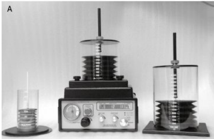
Figure 5.13. (A) Example of a standing (ascending) bellows configured ventilator with a plate system that can be used to limit the tidal volume. Alternatively, the tidal volume can be limited by adjusting the inspiratory gas flow and/or inspiratory time. Courtesy of Mallard Medical, Redding, CA. (B) Schematic of generic dual circuit ventilator demonstrating the gas flows within the ventilator during inspiration and expiration. Note that the exact position and design of various components varies among manufacturers. Illustration by Kath Klassen, BSc (Agr), DVM.
