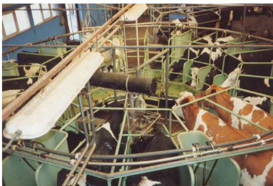
Fig. 8.18. Rotary parlour, with cows on a turntable that rotates once for each cow.
