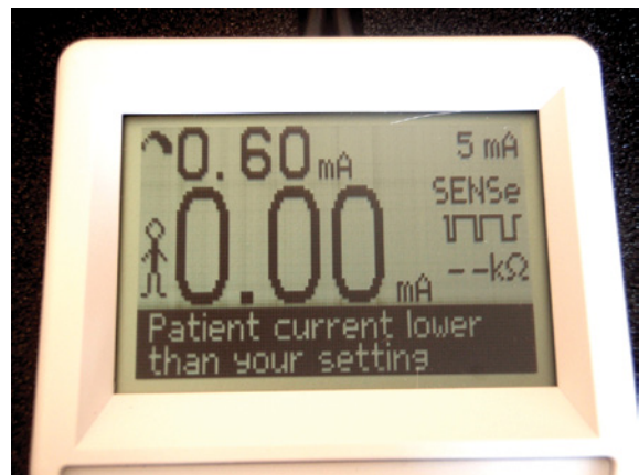
Figure 6.6 Example of a nerve stimulator (Stimuplex® HNS12, B.Braun Medical Inc.) with LCD display that presents a warning message when the delivered current is not the same as the set current.
