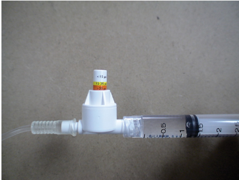
Figure 5.17 An inline pressure gauge (BSmart™, Concert Medical) can be used to monitor injection pressure during performance of regional anesthetic nerve blocks. Note the color-coded piston that relays objective information about the pressure being applied to the patient's tissues during injection of the local anesthetic solution.
