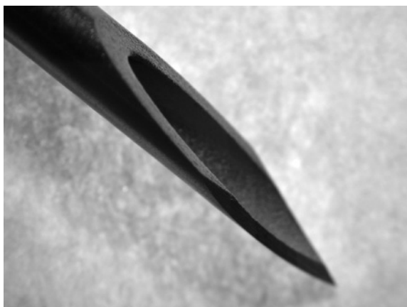
Figure 5.1 The tip of an 18-gauge hypodermic needle bevel viewed at 25 \times . Hypodermic needles have a long bevel and sharp edge and are specifically designed for puncturing skin and adjacent tissues. Note the long bevel (15°) and sharp cutting edge of this needle.
