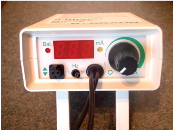
Figure 6.7 Example of a nerve stimulator (Stimuplex® Dig RC, B. Braun Medical Inc.) with a digital display, adjustable impulse frequency (1–2 Hz), and adjustable current (mA).
