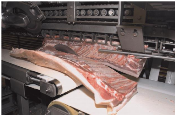
Figure 4 View of splitting the middle into the loin and belly in the automatic cutter for pork middles. Photo courtesy of Attec.
