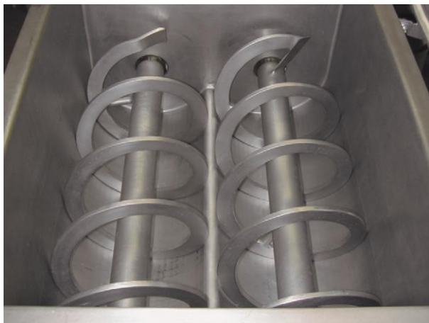
Figure 2 The same mixer as shown in Figure 1 fitted with twin ribbons to function as a ribbon blender.
