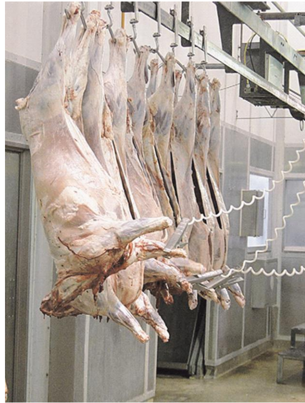
Figure 5 A low-voltage stimulation unit for sheep that can be used in processing plants with a small throughput. The current (80 V peak, 120–300 mA peak, 15 pulses per s) passes from the front legs to the earthed rail. The duration of stimulation ranges from 30 to 60 s. In this system, the stimulation is applied at the end of dressing but earlier stimulation at the end of stunning may be used and this has the advantage that carcass movement poststun is reduced. Three sheep are connected at a time in this system. The carcasses with the current flowing have the front legs outstretched.
