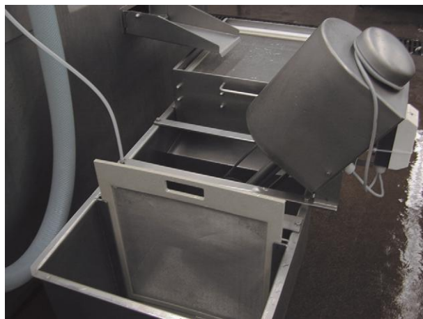
Figure 5 An accumulator tank. Note the filter screens and the pickle agitator.
