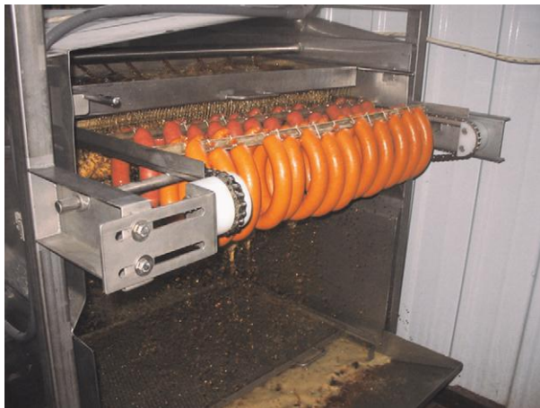
Figure 2 Showering or drenching the surface of the meat product or immersion in smoke condensate solutions is widely used. In drenching, a solution of the smoke condensate is showered over the product for a specific amount of time. Normal solution concentrations range from 5% to 50% smoke. The smoke condensate solution is recirculated through a filter system and back over the product to get the highest usage out of the condensate. The meat products are showered for 15–90 s to obtain the desired results (see Table 2 for an example of a showered frankfurter processing schedule).
