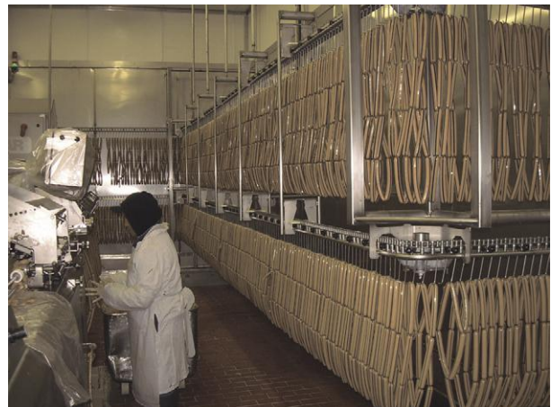
Figure 6 Horizontal serpentine chain-and-hook conveyor – continuous small sausage cook/chill system. Linked sausages are automatically looped onto hooks attached to a chain. Reproduced with permission of Marathon Enterprises, Inc., USA.
