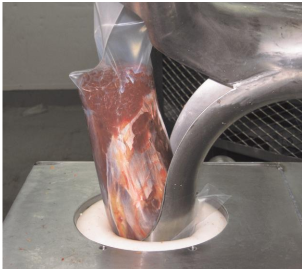
Figure 6 Stretched beef being ejected from the flexible sleeve into the packaging. Photograph courtesy of D.L. Hopkins.
