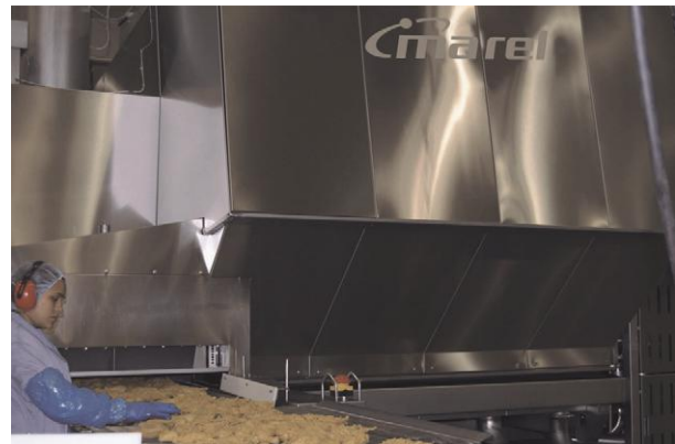
Figure 10 Spiral-belt continuous oven. Product is conveyed on a belt that is configured as one or more spiral towers. Airflow is horizontal across the belt and parallel to the product. Reproduced with permission of Marel Townsend Further Processing, USA.
