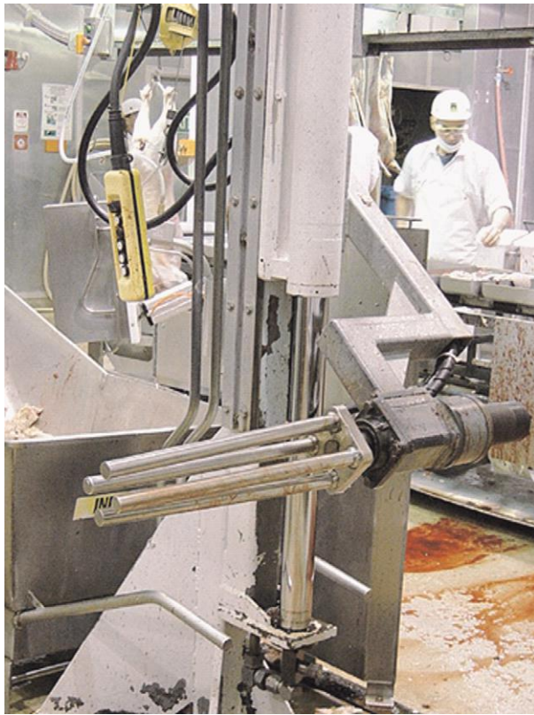
Figure 3 The four prongs are part of a system to remove the pelt from a sheep carcass. The pelt is freed from much of the carcass, and a hanging portion is placed between the prongs, which can rotate.
