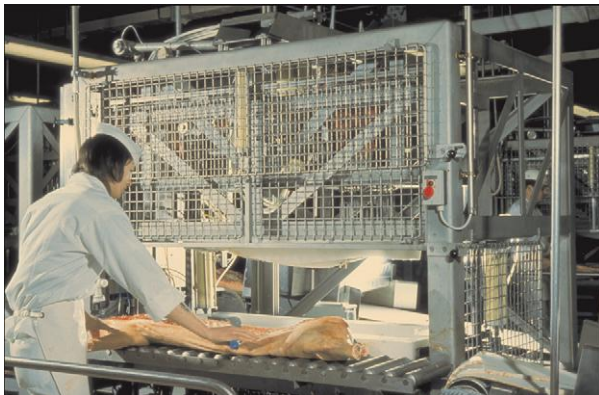
Figure 3 From 1970 to 1986 Danish bacon sides for Britain were injected using a special machine in which 109 needles injected the brine evenly from both the meat and rind sides into the muscles. Nowadays, it is common practice to use continuous multineedle injectors for the production of bacon cuts.
