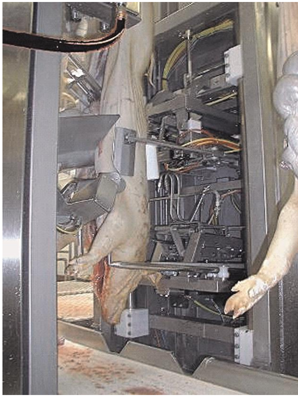
Figure 3 Automatic evisceration. The automatic evisceration machine cuts the diaphragm, tears off the flare fat, and loosens the intestinal tract such that the entire set of intestines and organs is removed from the carcass before separation (Anon, 2001a,b). Because the separation takes place outside the carcass, it can be performed consistently and reliably with lower risk of fecal contamination.
