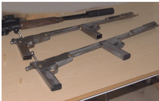
Figure 5 Two modified weapons used for stunning bulls and cows. The original weapon is shown above and the two weapons below have been modified to activate the firing of the bullet only when the trigger is pressed and the rod under the muzzle is pushed in when placed on the animal's forehead.
