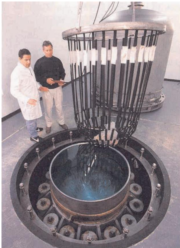
Figure 10 A large-scale Hydrodyne unit (1060 l) showing the inner section where the encased meat and surrounding water are held, with the large dome in the background. Photograph courtesy of M.B. Solomon.
