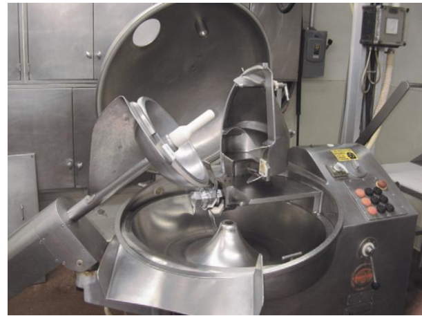
Figure 5 A bowl chopper fitted with a vacuum hood. The knife hood is open to show the six-blade knife assembly. The unloading scoop is to the left of the knife assembly.
