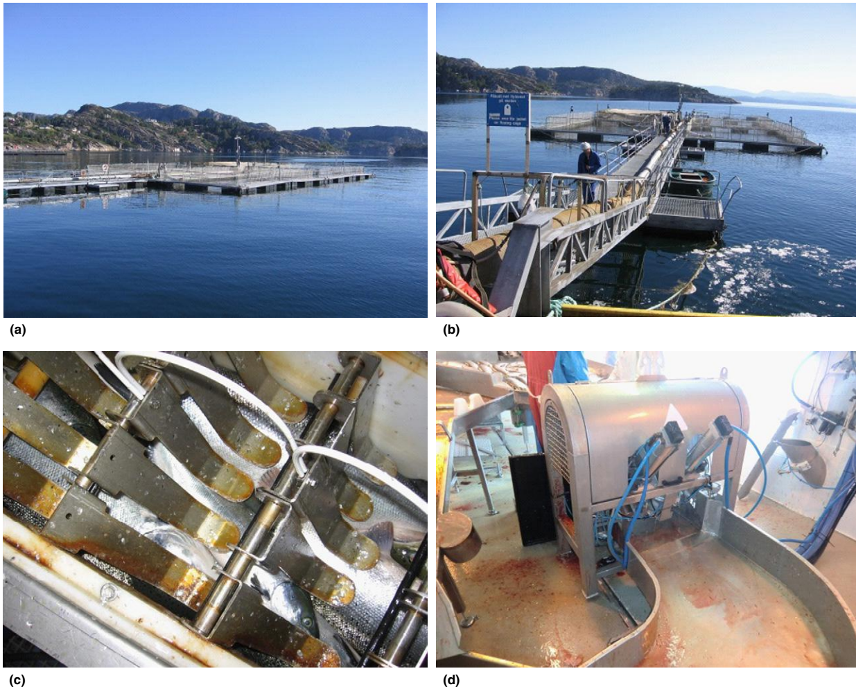
Figure 1 (a) Stunning and killing of Atlantic salmon: lairage, (b) pumping of fish to the slaughter facilities, (c) electrical stunning after draining the water, and (d) killing the stunned fish by percussion and gill-cutting.
