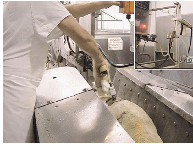
Figure 1 A slaughterman applying a head-to-back stun to a sheep in a restraining conveyor. Inset: A stun gun showing the pointed front electrodes that are applied to the head and the flat rear electrode through which water is also applied to the wool to lower electrical resistance.
