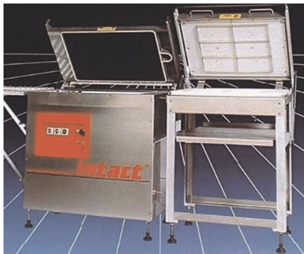
Figure 7 Vacuum skin packaging machine. Trays of meat are placed on magazine (right) before being placed in chamber. Barrier film is softened by a heating element in lid before being molded to trays below. Reproduced with permission from Cryovac Sealedair Corporation, Hamilton, New Zealand.
