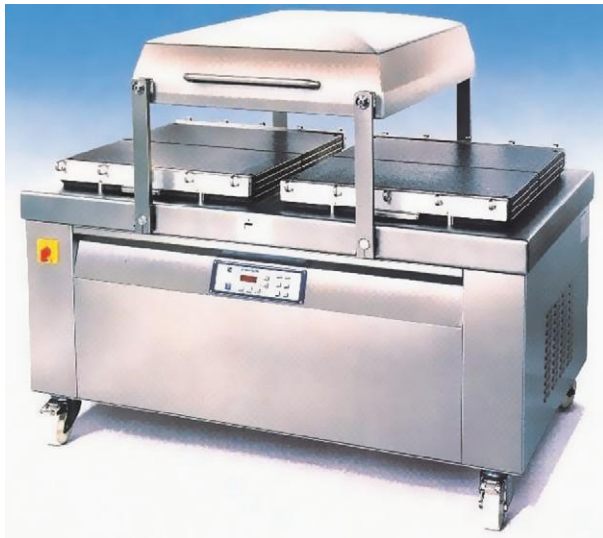
Figure 3 Twin vacuum chamber machine. Meat in oxygen-barrier bags is placed on one platform. The chamber hood is lowered, a vacuum is applied within the chamber, and the vacuum-barrier bag is sealed and the chamber is vented. Reproduced with permission from Cryovac Sealedair Corporation, Hamilton, New Zealand.
