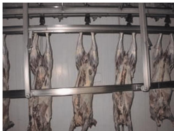
Figure 4 A typical high-throughput system using a high voltage ES facility for sheep postdressing, in which the current passes through the carcass between two rubbing bars. Photograph courtesy New South Wales Primary Industries, Australia.
