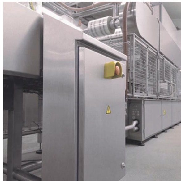
Figure 5 Hygienic design is a necessity for easy-to-clean production systems in hygiene-critical processes in the food industry. Reproduced with permission from Schmitt, H., Koch, H.R., 2011. Hygienic Design of Enclosure Boxes in Relation to High Pressure Cleaning?
