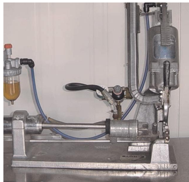
Figure 2 Hand-operated Clippertie vacuum clip system. Meat product packaged in oxygen barrier is sealed with a metal or plastic clip (contained in the reverse-J-shaped formation) around the gathered packaging material.
