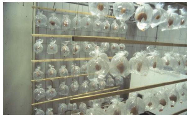
Figure 1 Illustration of the gravimetric method for measuring drip loss, involving suspension of a meat sample in an inflated bag and storage at 2\text{--}4^\circ\text{C} for 1–2 days. Credit: Kaufman, R., University of Wisconsin–Madison.
