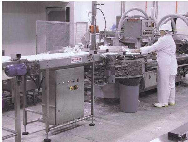
Figure 4 Rotary vacuum chamber machine. Meat in oxygen-barrier bags is placed on conveyor at the left and fed into one of many vacuum chambers for evacuation and sealing. Reproduced with permission from Cryovac Sealedair Corporation, Hamilton, New Zealand.
