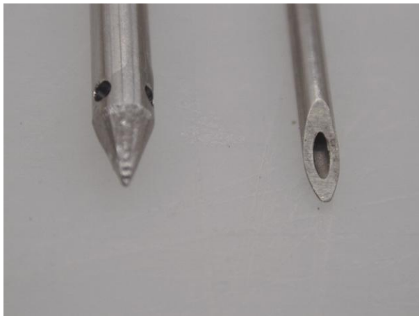
Figure 4 Injector needles. Left, a side-port needle; right, a hypodermic-type needle.
