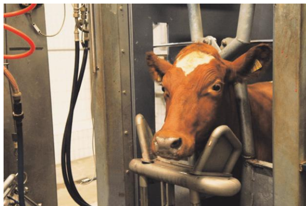
Figure 7 A restraint device for pneumatic stunning of cattle using both neck restraints and a chin-lift.
