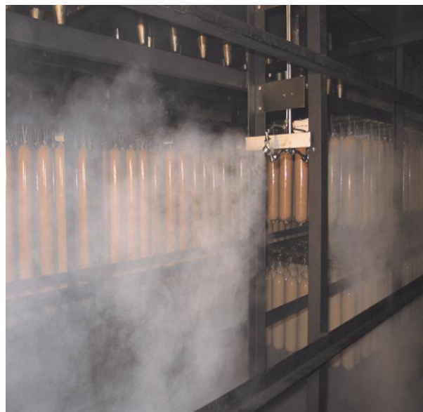
Figure 1 Smoke application in a smoke chamber is carried out with low-velocity circulating air or air movement derived only from the application mechanism itself. The amount of smoke applied is controlled with metering pumps or by air pressure. Optimal smoke regeneration is obtained by sequential steps that include an atomization step followed by a circulation step while the dampers of the smoke house are closed. This also optimizes the use of the smoke. Multiple cycles of smoking and circulating may be utilized to provide the desired flavor and color (see Table 1 for an example of a frankfurter processing schedule with condensed smoke regeneration).
