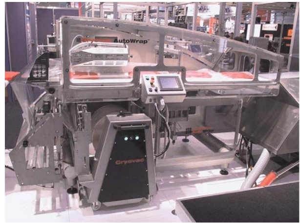
Figure 5 Flow wrap. Flexible-barrier film is passed through a former (on the left of figure), producing a tube around the meat (center) before vacuuming and sealing. Reproduced with permission from Cryovac Sealedair Corporation, Hamilton, New Zealand.
