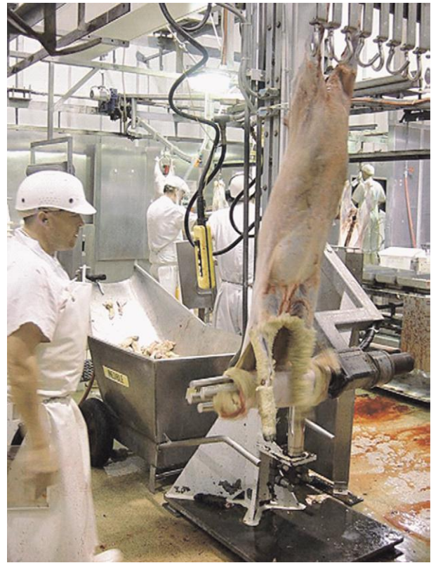
Figure 4 The rotating prongs grip the pelt and pull it down over the rear legs in this inverted dressing system.
