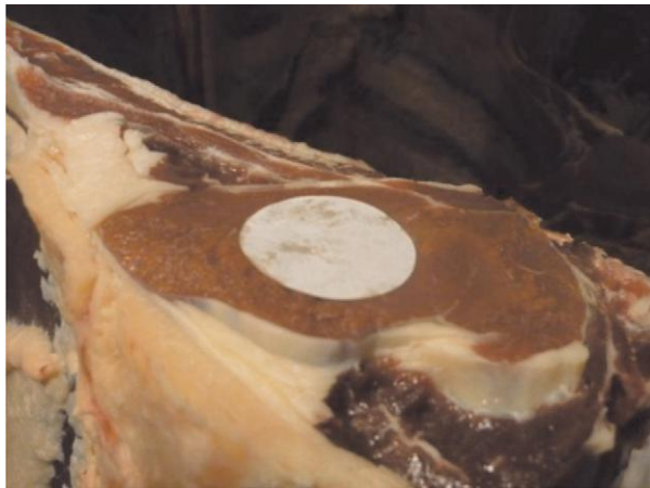
Figure 3 Illustration of the rapid filter method for measuring weep or exudate on a beef loin surface. The filter paper can either be weighed, for amount of fluid absorbed, or be scored for percentage of wetness. Credit: Athula, N., Department of Primary Industries, VIC, Australia.
