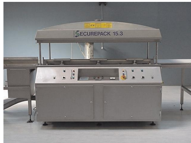
Figure 11 CAPTECH machine. Meat is placed in very high-barrier bags. The open end of the bags is placed over one of the three internal snorkels. The chamber is lowered, a vacuum is applied, and the storage atmosphere containing carbon dioxide is injected into the pack before sealing. Reproduced with permission from Securefresh Pacific Ltd., Auckland, New Zealand.
