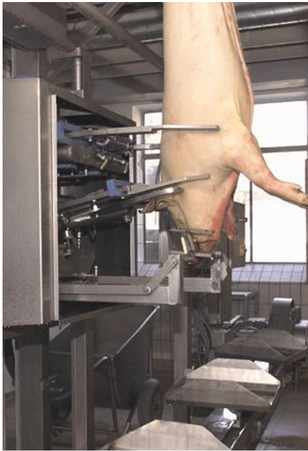
Figure 5 Head-cutting machine. The machine operates in two modes. It can either cut off the head entirely or leave it on a separate conveyor system or alternatively the machine can cut the neck only and leave the head hanging at the carcass by the jowls. Cutting off the head before carcass-splitting reduces the risk of contamination from the mouth and throat regions. The machine also provides better yield by leaving more neck meat on the carcass.
