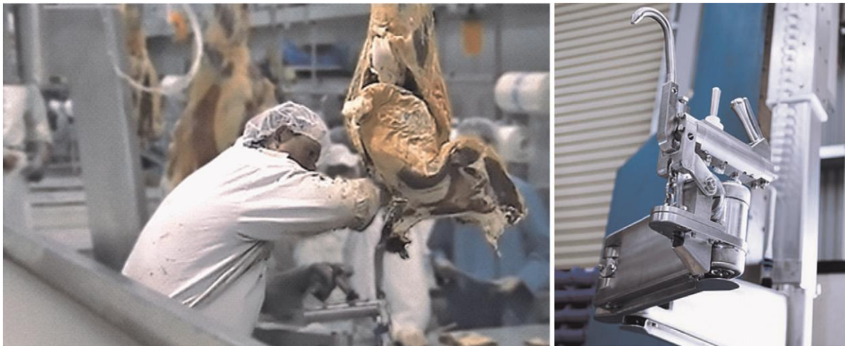
Figure 7 An adaptive controlled pulling device called Hook assist developed in an MLA/AMPC and Scott effort. Photo courtesy of Scott Technology Australia P/L.
