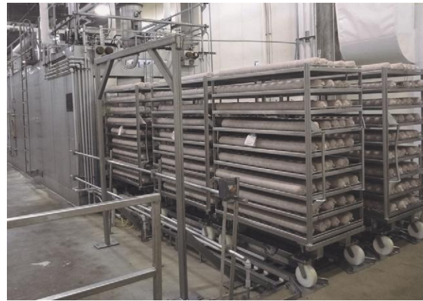
Figure 9 Floor-mounted walking beam conveyor – continuous steam-cook/brine-chill system for molded hams. Hydraulic cylinders are used to index the loaded racks through the system. Reproduced with permission of Butterball LLC, USA.
