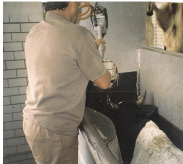
Figure 1 Well-designed stun box that is the correct width to prevent animals from turning around. A common mistake is to make stun boxes too wide. Stun boxes must have nonslip flooring. Animals remain quieter on nonslip flooring.
