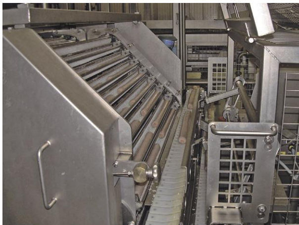
Figure 8 Serpentine chain-and-tray conveyor – continuous coextruded sausage system. Blended sausage meat is coextruded with collagen dough to form continuous ropes of sausage encased in a film of collagen dough. Ropes are automatically cut to length, and cut sausages are loaded into trays that span the gap between two chains. Reproduced with permission of Salm Partners LLC, USA.
