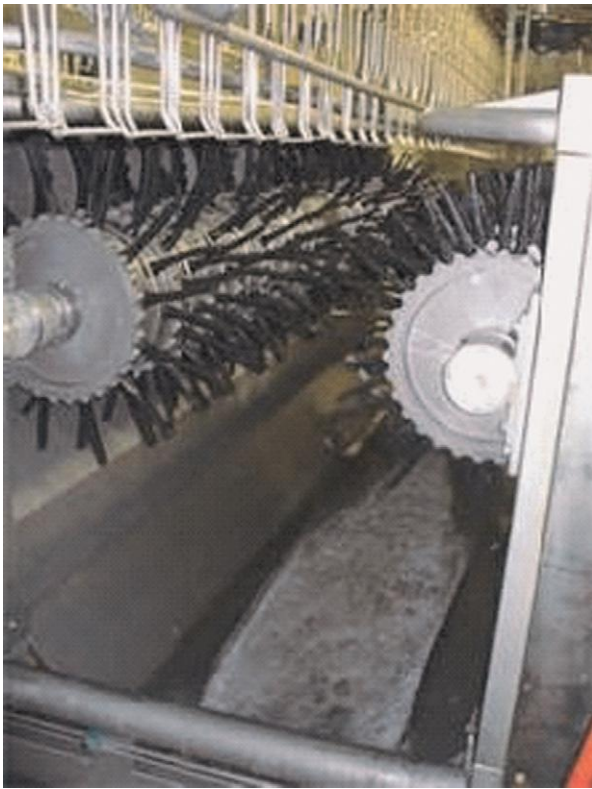
Figure 3 Side view of rubber fingers mounted on rotating disks and used for picking/plucking poultry feathers.
