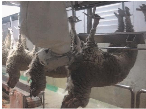
Figure 7 IRL's Y-cut robot opens the pelt inside each leg. Photo courtesy of Callaghan Innovation, formerly IRL, and Ovine Automation Limited.
