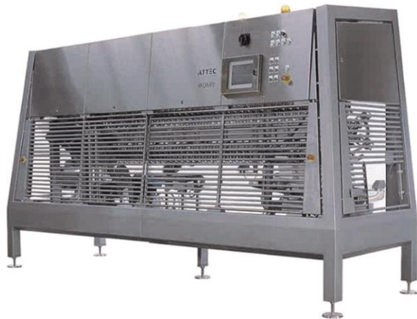
Figure 2 Automatic cutter for pork middles. Photo courtesy of Attec.
