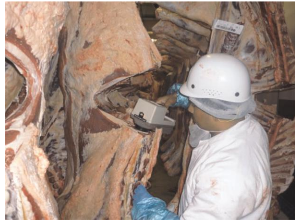
Figure 7 A portable Hunter Mini Scan instrument (Model 45/0-L) being used in the field to measure percentage reflectance on an exposed beef loin muscle. The muscle has been exposed to the air for 30 min and is done after rigor is completed. This machine is not used for grading purposes but certainly has potential to be used in this manner. Credit: Athula, N., Department of Primary Industries, VIC, Australia.
