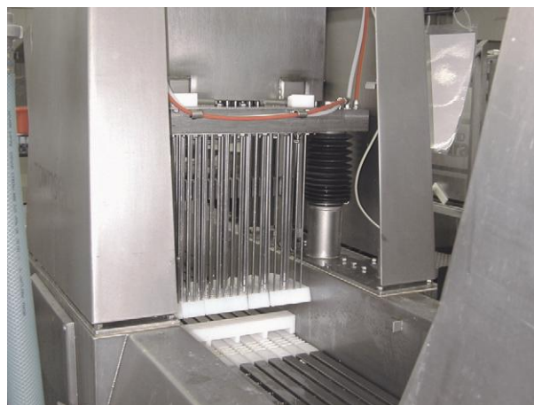
Figure 1 A bone-in injector with the cover open to show the multiple-needle injection head.
