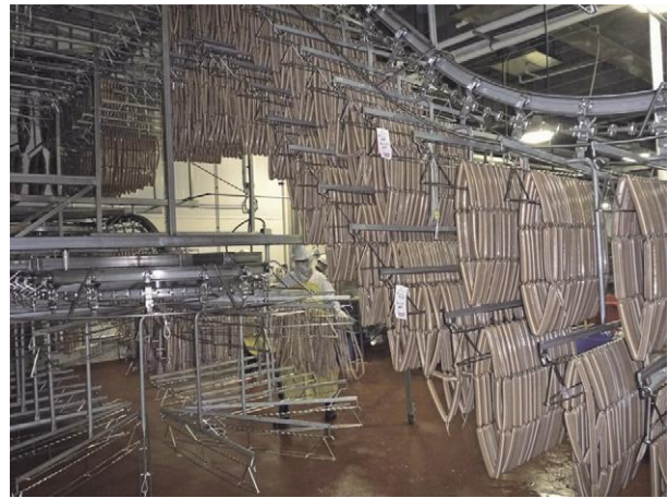
Figure 5 Horizontal serpentine chain-and-yoke conveyor – continuous small sausage cook/chill system. Linked sausages are looped on sticks and then sticks are manually hung on yokes attached to a mono-rail chain conveyor. Reproduced with permission of Maple Leaf Foods, Inc, Canada.
