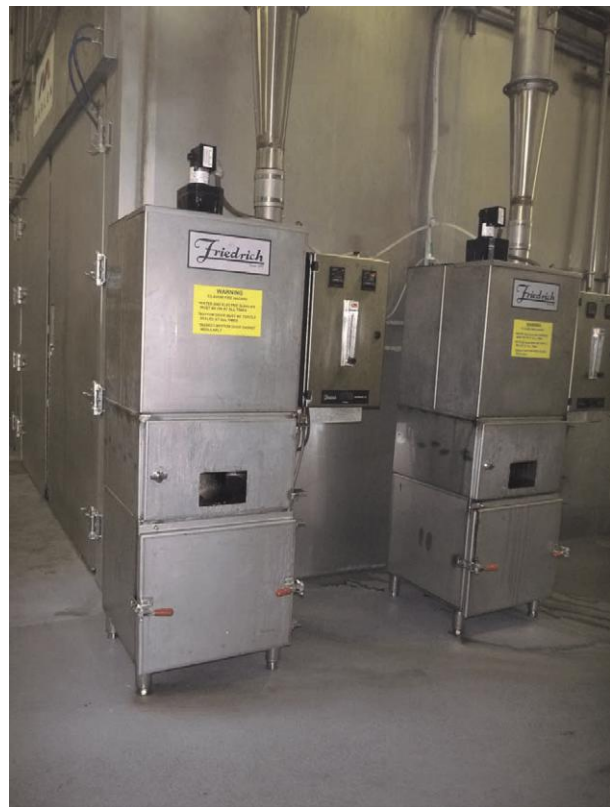
Figure 15 Dry-sawdust hot-plate smoke generator. Reproduced with permission of Villari Brothers Foods LLC, USA.
