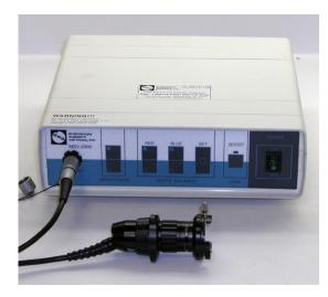
FIGURE 1-3. Endoscopic video camera.
