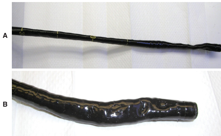
FIGURE 1-44. A and B, Crush damage to the distal end. Caused by accidentally entering the scope into the oral cavity during gastroscopy.
