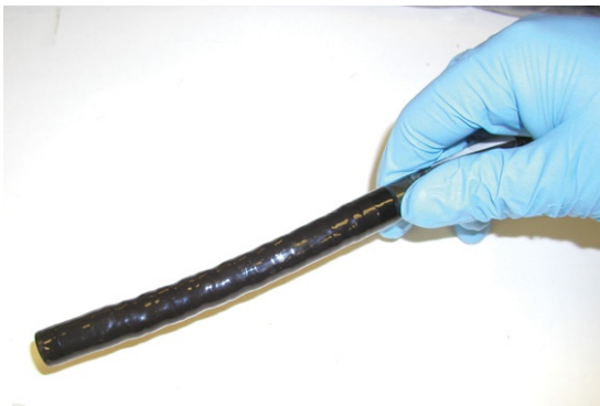
FIGURE 1-14. Inspecting flexible bending rubber.
