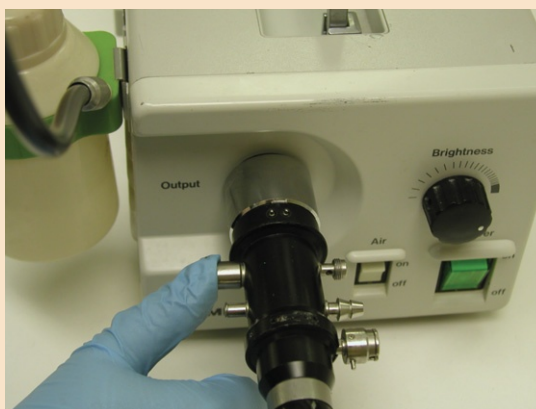
FIGURE 1-38. Depressing water valve.
