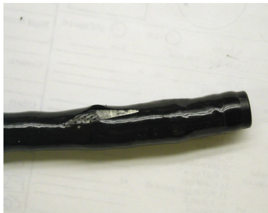
FIGURE 1-41. Torn bending rubber.
