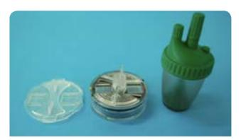
Figure 7. Devices in the "FLOTAC family": Mini-FLOTAC, FLOTAC and Fill-FLOTAC.
