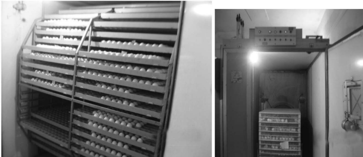
Fig. Setter and Hatcher for artificial incubation of eggs
