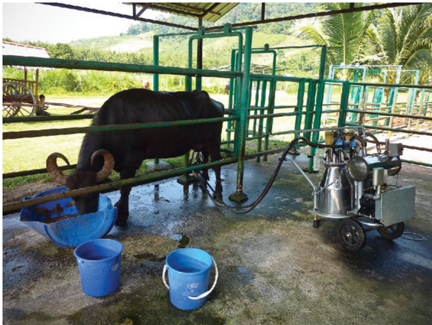
Plate 3.2. Buffalo milking with autonomous bucket machine milking.
