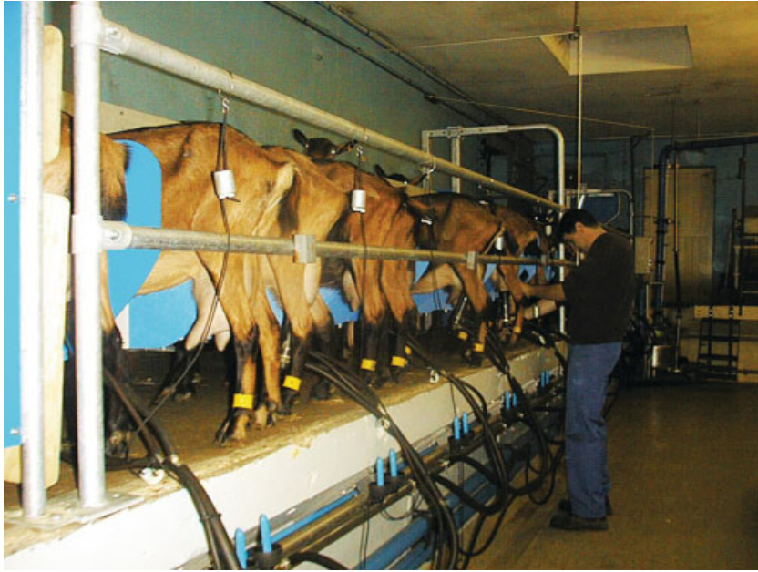
Figure 3.1. Simple platform, side-by-side, milking parlor for goats at the AGROCAMPUS OUEST/INRA laboratory. For a color version of this figure, see Plate 3.1.
