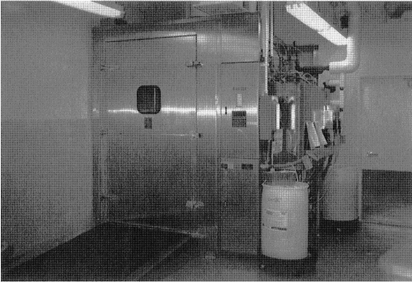
FIG. 4. Mechanical cage washing equipment for thorough sanitation.
