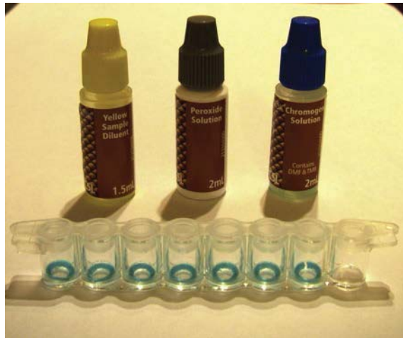
Figure 7.7. Commonwealth serum laboratories (CSL) snake venom detection kit (SVDK): detection of tiger, brown, black, death adder, and taipan envenomation with +ve and –ve controls and blank well. The SVDK available in Australia enables the detection of snake envenomation using blood, urine, or a swab from the bite site. It also allows identification of the type of snake (which may influence treatment and prognosis). It is advised to perform test on cat heparinized blood or plasma (preferable) if envenomation occurred less than 8 h prior to presentation and to use urine if the time post envenomation is greater than 8 h or unknown.
