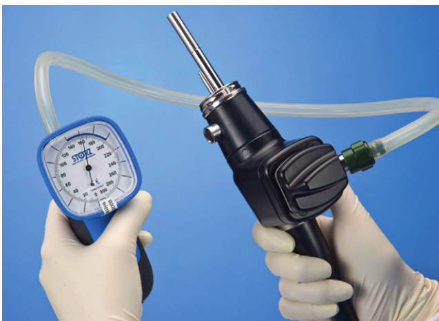
Figure 27-4 Manometer for testing leakage of the endoscope.
