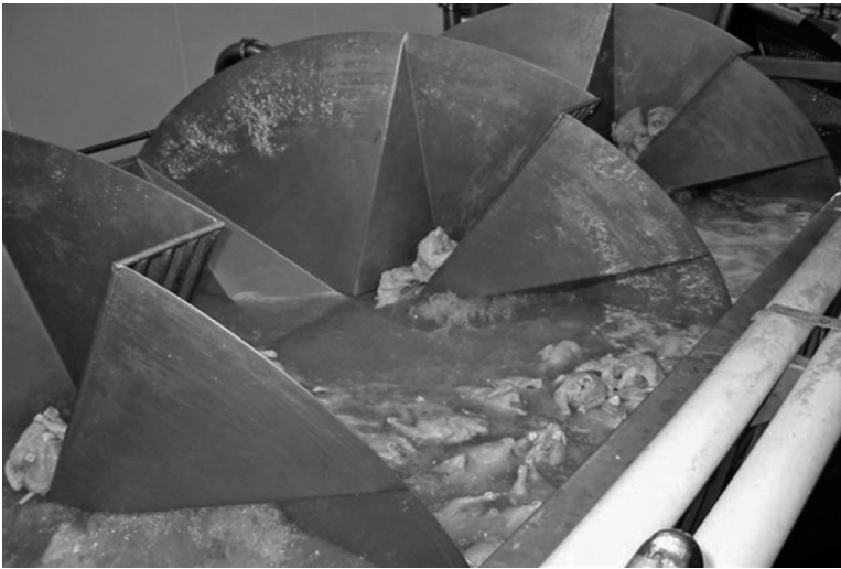
Figure 21.6 This is a chiller in El Salvador that is operating properly with extremely clean water containing very low organic loading.
