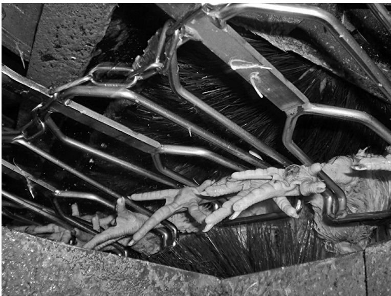
Figure 13.5 Inside view of a prescald bird brush system.
