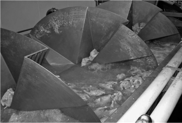
Figure 28.2 Typical immersion chiller used in the United States.
