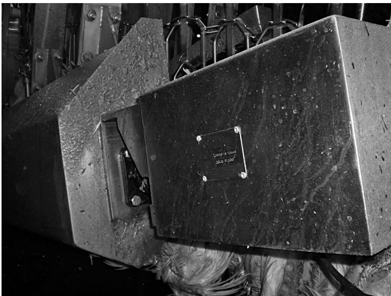
Figure 13.4 Outside view of a prescald bird brush system.
