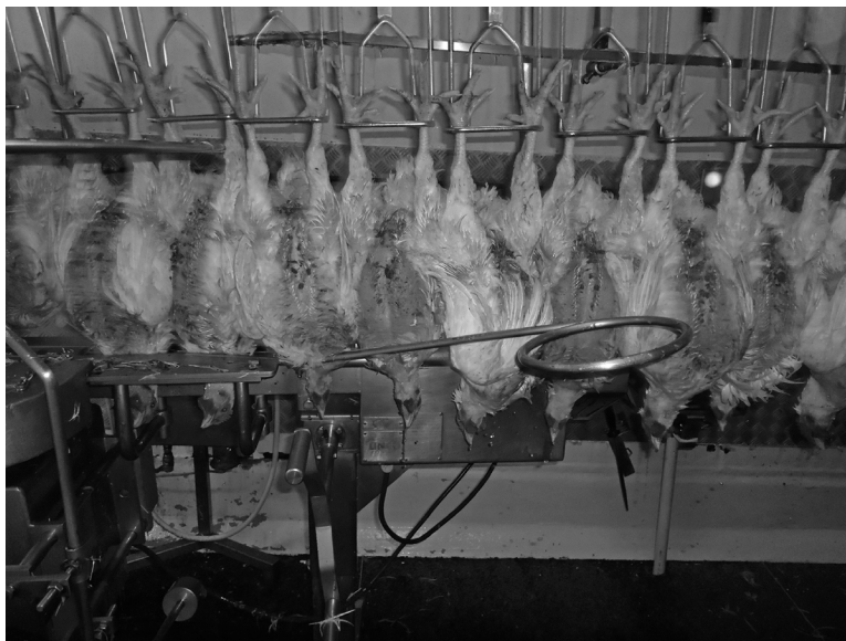
Figure 13.2 Excessive fecal material clumped onto the breasts of live chickens before scalding.
