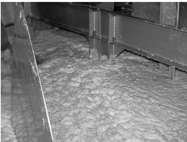
Figure 21.4 Another example of the exit of a chiller with water containing high levels of fat due to overscalding.
