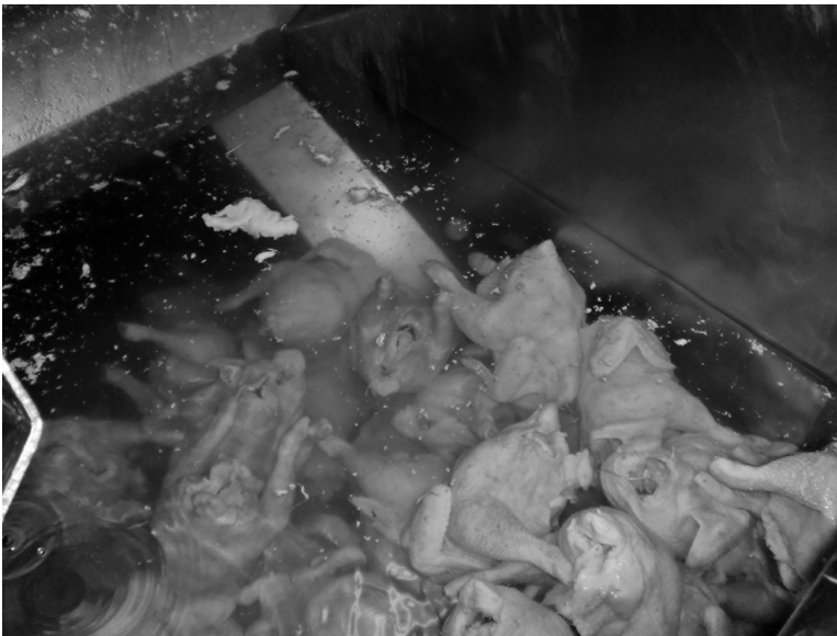
Figure 21.7 This is a chiller in Chile that is operating perfectly with extremely low organic loading at the chiller exit.
