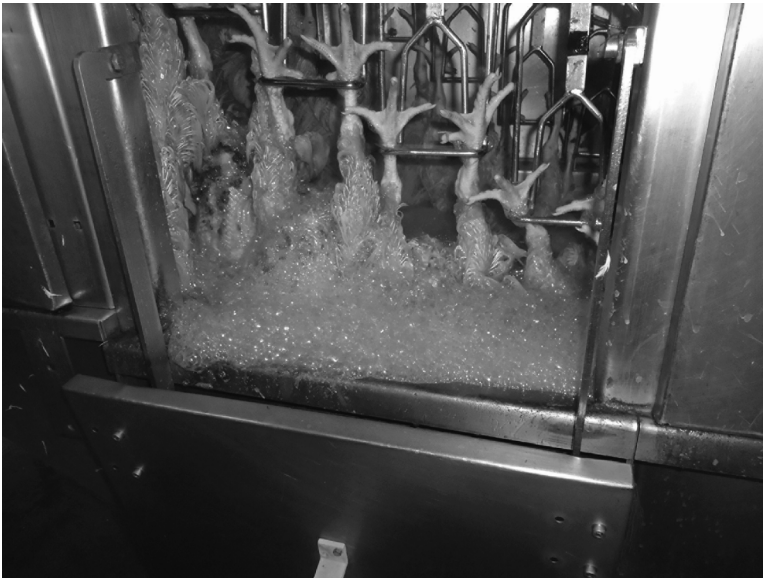
Figure 13.10 A scalding tank that is not operating in a countercurrent fashion showing filthy scald water and clumped fecal material on carcasses.
