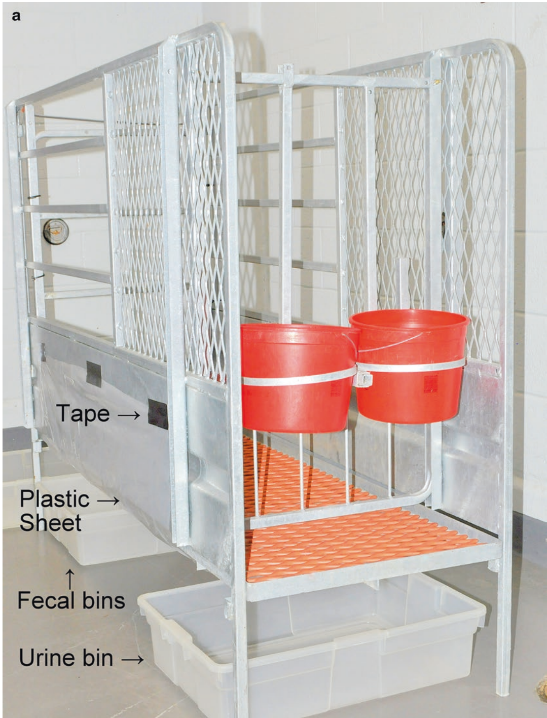
Fig. 1 (a) Elevated calf stall depicting urine collection bin and plastic urine diversion sheet placement, viewed from front. (b) Stall depicting fecal collection bins and plastic urine diversion sheet placement, viewed from rear. (c, d) Newborn 41 kg Holstein bull calf in stall ~1 h following arrival at ABSL-2 facility, prior to infection
