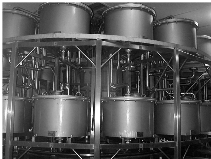
Figure 5.8 Continuous ion exchange chromatography plant for processing cheese whey at an Australian dairy company (see also De Silva et al., 2003). Reproduced with permission of CSIRO.
