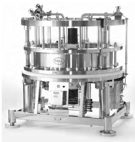
Figure 5.1 An example of a batch chromatography column is the “Resolute” column manufactured by Pall Corporation. This has a three-position nozzle valve to enable packing, unpacking, and running of the column. Provided with compliments of Pall Corporation. Copyright Pall Corporation, 2010.
