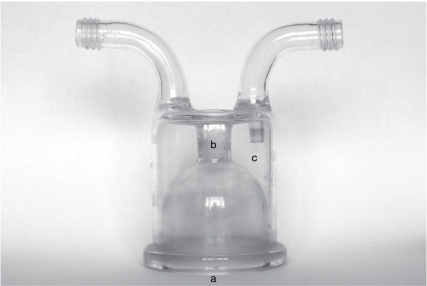
Figure 9.2 Rutledge-type feeder. The Rutledge feeding system consists of a jacketed hollow cone, the base of which can be covered by an artificial membrane or animal skin (a). Blood is introduced into the cone through a tube (b) that extends from its
