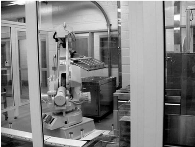
Fig. 12-8 Robotic cage-washing system showing both the soiled-side robot (left) and clean-side counterpart (right). The soiled side also shows the dirty bedding dumping station (D), in conveyor track (I) and first tunnel washer section (T). On the clean side are bedding cages on the out conveyor (O), automated bedding dispenser (B) and egress section of the tunnel washer (T).
