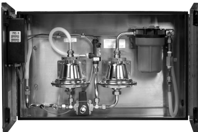
Fig. 32-1 Pressure-reducing station. The canister at the right within the PRS contains a 5.0 micron particulate filter; the two silver structures on the left and in the center are the valves that control the pressures for normal drinking and for system flushing.
