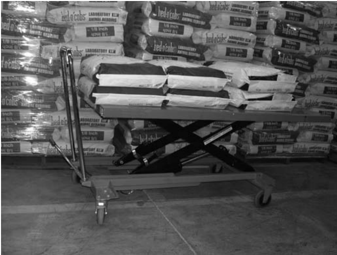
Fig. 12-4 Adjustable (scissors) dunnage rack allows for the loading and unloading surface to be adjusted as needed to the safe height for any worker. Photograph courtesy of Emory University, Atlanta, GA.
