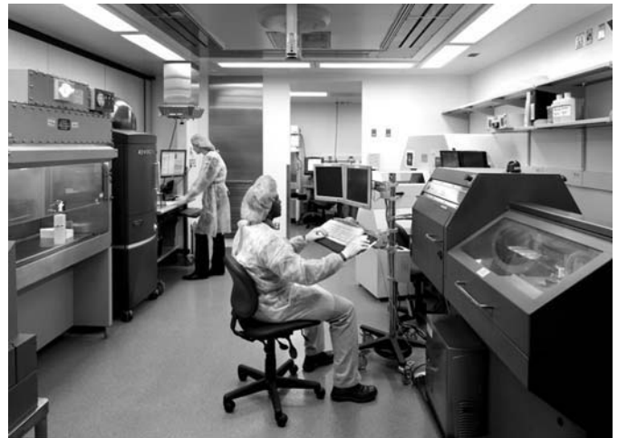
Fig. 20-7 A rodent-imaging laboratory containing various types of imaging equipment and support equipment. A combination SPECT and CT scanner is present in the right foreground, a microCT scanner is in partial view, a biological safety cabinet is located in the left foreground, and an optical imaging system can be seen in the left background.
