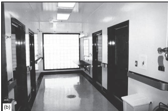
Fig. 19-11 (a) Animal holding suite with procedure laboratory. (b) Suite vestibule. This is an entry vestibule into four rooms (one procedure laboratory and three animal holding rooms). Suite arrangements allow for compartmentalization of compatible studies to utilize shared procedures laboratories.
