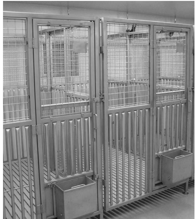
Fig. 22-2 Stainless-steel runs constructed of a combination of tubular materials and mesh on the upper panels with raised fiberglass slat flooring panels. The runs are 4' × 6' in dimension with sliding gates between the runs allowing for pair- or group-housing of adjacent animals as needed. The room is configured for wet sanitation with a trench drain and flush mechanisms (not visible) located behind the runs and a central ceiling-mounted hose reel.
