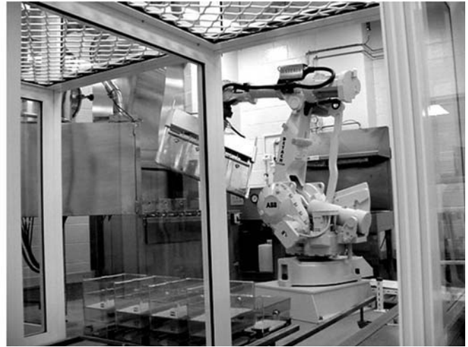
Fig. 12-8 Robotic cage-washing system showing both the soiled-side robot (left) and clean-side counterpart (right). The soiled side also shows the dirty bedding dumping station (D), in conveyor track (I) and first tunnel washer section (T). On the clean side are bedding cages on the out conveyor (O), automated bedding dispenser (B) and egress section of the tunnel washer (T).
