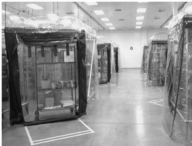
Fig. 20-25 Multiple portable, positive-flow/pressure, flexible-wall, vertical-flow MAD rooms for mouse holding and breeding.
