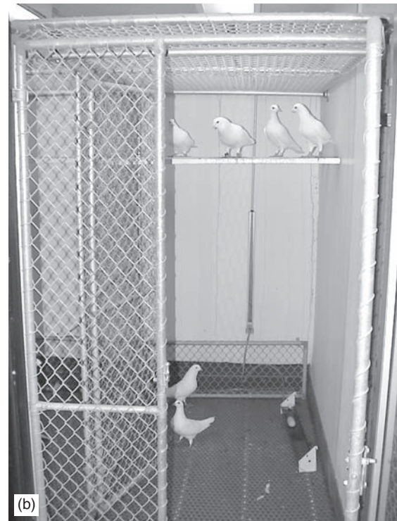
Fig. 15-17 Large animal cubicles housing birds, showing that they are useful for more than housing large laboratory animals.
