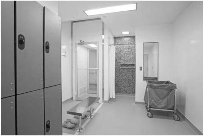
Fig. 18-9 The gowning area for entry into a barrier. Lockers are seen in the foreground and a shower is in the back right. In the center of the picture is a step-over bench where shoe coverings are donned, and beyond that is the air-shower entry into the barrier.
