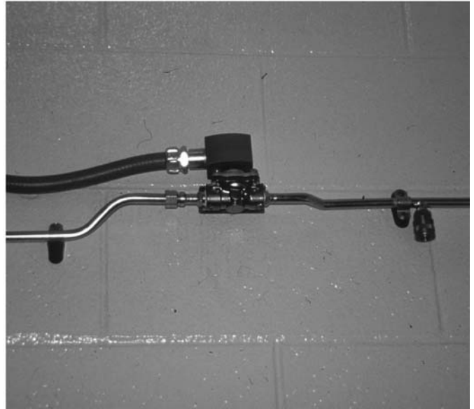
Fig. 32-11 Solenoid valve on a non-recirculating system. Electronic activation of this valve enables higher-pressure water to flush through the system to reduce biofilm development.
