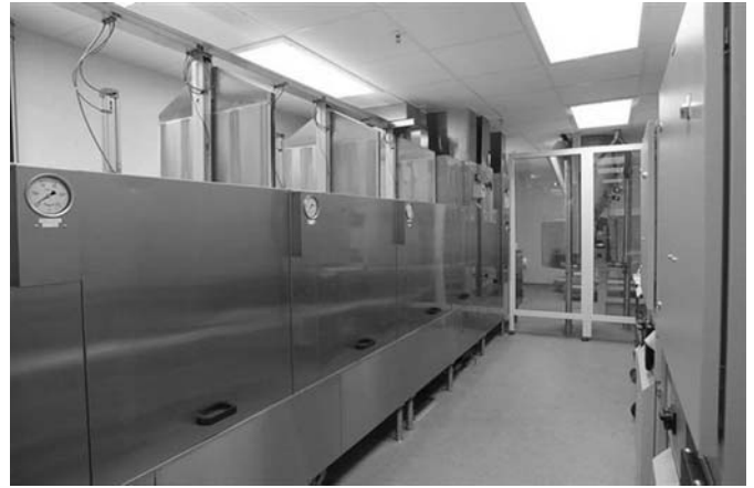
Fig. 31-15 Indexing tunnel washer. Note retracting panels above machine to create closed sections of tunnel washer.
