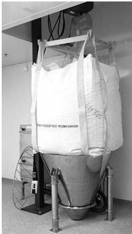
Fig. 12-5 Overhead emptying of a bulk bag of contact bedding into a bedding system load funnel enabled by a hoist and rail overhead system. Photograph courtesy of Detach AB, Strängnäs, Sweden.
