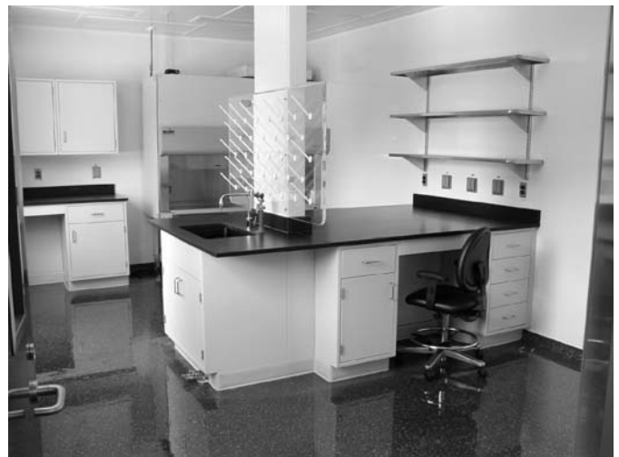
Fig. 16-9 A typical laboratory with installed cabinetry, sink, and a biological safety cabinet.
