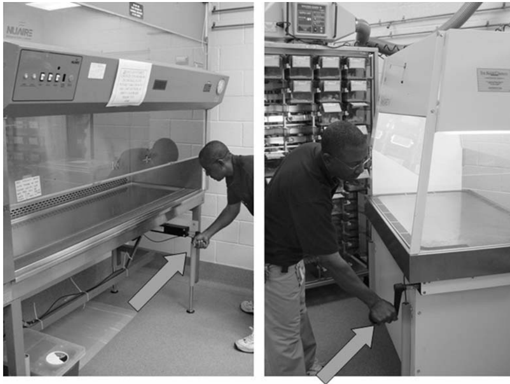
Fig. 12-6 Stationary biosafety cabinet (left) and mobile cage-changing station (right) featuring front grills of minimal depth to decrease reaching and stretching to areas of the work surface and height adjustability by hand-crank (arrows). Automated hydraulic lifts are an option instead of manual cranks. These features allow for safe postures and reaches to be used by a range of workers of varying height and size.
