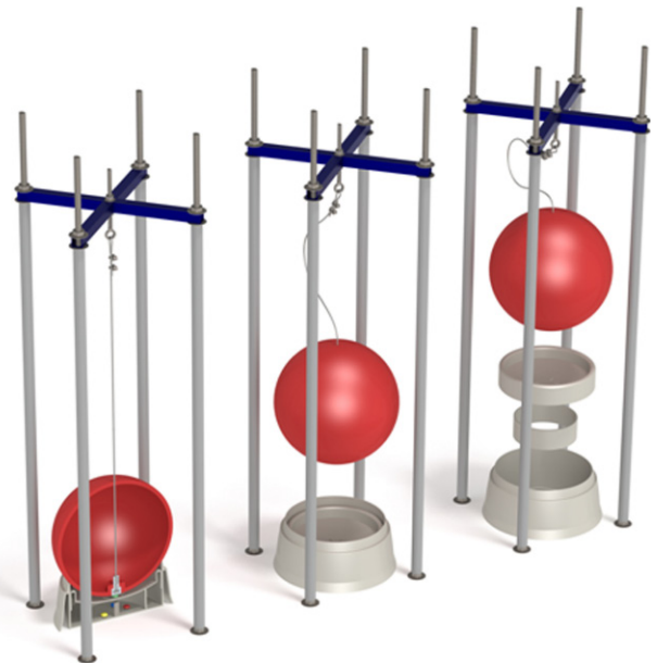
FIGURE 39.2 Details of the “holes” used in both the pig holeboard setup and the active choice setup used in judgement bias and decision making. Plastic balls are fitted with magnets and hung from a stainless steel wire in between four stainless steel rods. The balls lay in plastic dishes which contain sensors that can detect movement of the magnet. When the animal displaces the ball, either to gain access to a reward or as an operant response, the sensor detects movement of the magnet, and sends a pulse through the interface to a computer running registration software. Source: Modified from Antonides et al. (2015a), according to Open Access terms.
