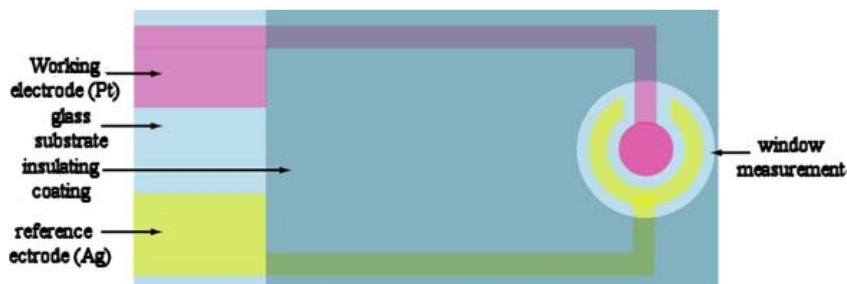
Figure 7. Schematic drawing of the micro-sensor.
