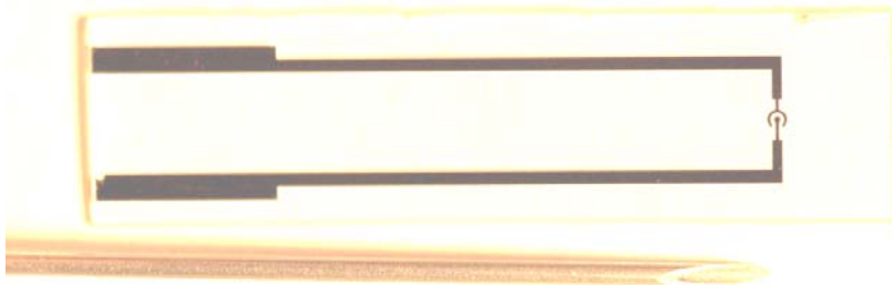
Figure 9. The micro-sensor realized by lift-off process.
