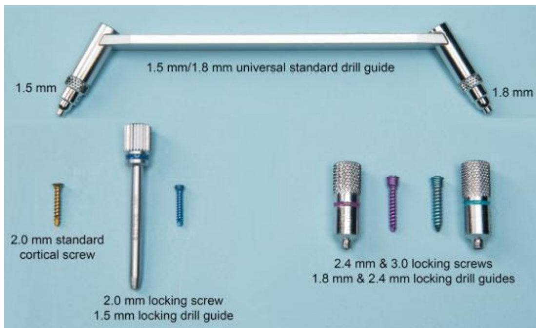
• FIG. 33.4 Instrumentation to apply the screws in the 2.0- and 2.4-mm plates. The standard universal drill guide with 1.5-mm and 1.8-mm drill sleeve diameters; the core diameter of the 2.0 mm-screw corresponds to a 1.5-mm drill bit, and the 2.4-mm screw corresponds to the 1.8-mm drill bit. The core diameter of the 2.0 locking screw also corresponds to a 1.5-mm drill bit; locking screw guide screws into the plate, which has threads within the screw hole, in order to center the drill hole within the plate screw hole, and in an orthogonal orientation. Similarly, the 2.4- and 3.0-mm screws have corresponding drill guides with 1.8-mm and 2.4-mm drill guides, respectively. Note that the screws and their respective drill guides are color coordinated.
