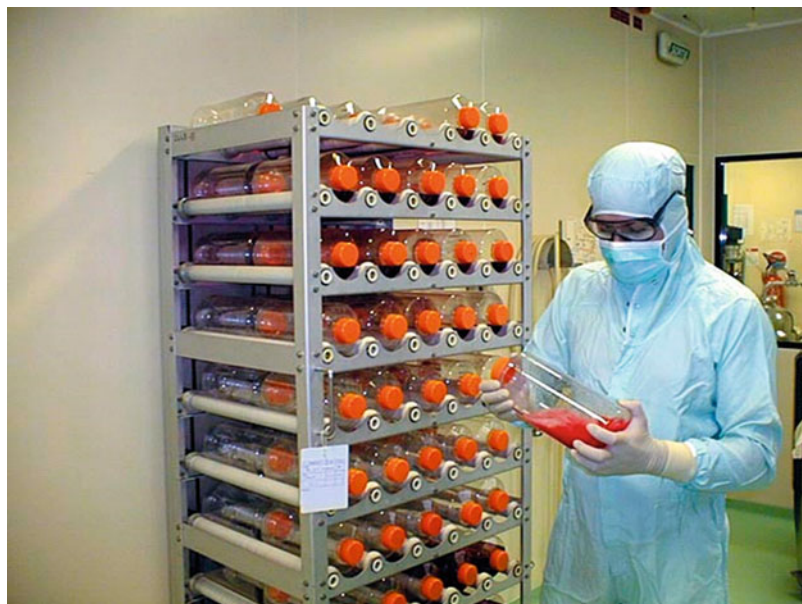
Fig. 1 Production of viral vaccines in monolayers in roller bottles
