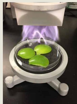
Here is a photo of a cold plasma jet treating apple slices, taken by Dr. Niemira
