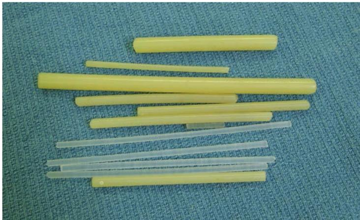
Fig. 10.9. Raw polypropylene rod stock.
