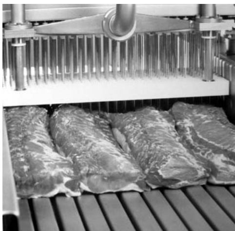
Fig. 15.1. Close-up of a brine injector with dense needle pattern. Source: P.H. Hoogenkamp.
