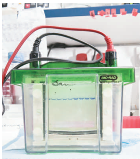
■ FIGURE 5.10 The experimental setup for gel electrophoresis. The samples are placed on the top of the gel. When the current is applied, the negatively charged proteins migrate towards the positive electrode at the bottom.
