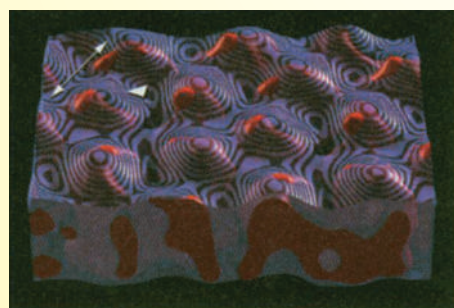
FIGURE 4A The AFM scan of the OmpF porin crystal in a membrane model. (From Native Escherichia coli OmpF porin surfaces probed by atomic force microscopy . F. A. Schabert, C. Henn, and A. Engel. (7 April 1995) Science 268 (5207), 92. Reprinted with permission from AAAS.)
