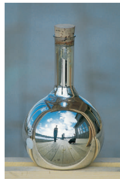
■ FIGURE 16.10 A silver mirror produced by an aldehyde. After the addition of Tollens reagent to an aldehyde, a silver mirror has been deposited in the inside of this flask.
