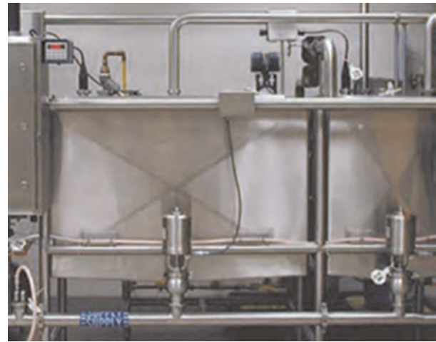
Figure 1 CIP cleaning solution and sanitizing solution tanks: This single use CIP system includes two medium-sized tanks for detergent and rinse/sanitizer, a steam heat exchanger, and programmable logic controllers to automate the cleaning process. Image courtesy of Ecolab.
