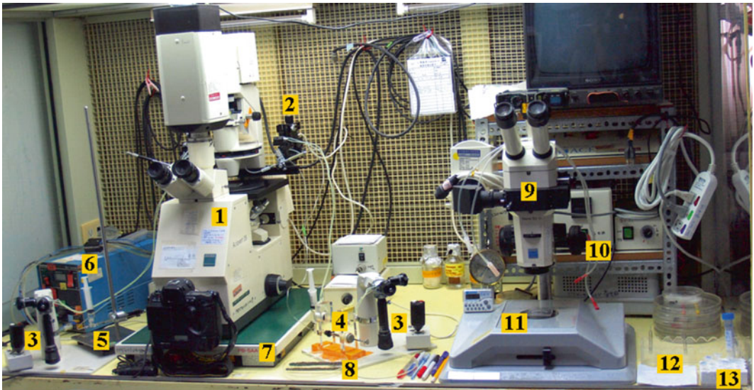
Fig. 2 The micromanipulation system and accessories have been used at my laboratory for more than 10 years. (1) A long working distance inverted microscope. (2) A motor-drive coarse micromanipulator. (3) A three-axis hanging-joystick oil-hydraulic micromanipulator. (4) A 500- \mu L screw-drive gastight glass syringe. (5) A laboratory-assembled 50- \mu L micrometer-drive gastight glass syringe. (6) A cooling device. (7) A portable anti-vibration table. (8) Homemade micropipettes secured on synthetic clay bars in a 100-mm cell culture dish. (9) A dissection microscope. (10) Mouth pipettes. (11) Homemade injection chamber. (12) Pipettes placing on an acrylic rack. (13) A 15-mL tube and 1.7-mL vials placing in a Styrofoam holder
