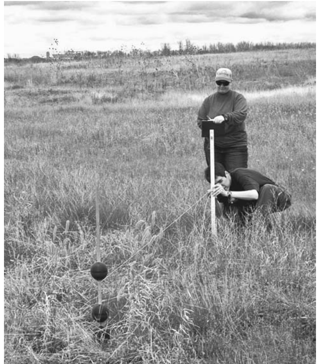
Fig. 16.11. Estimating horizontal cover using the staff-ball method of Collins and Becker (2001).
