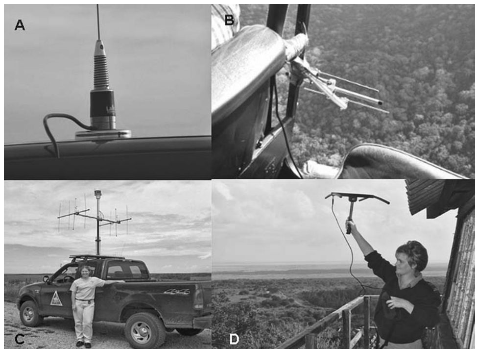
Fig. 10.5. Antennas for very high frequency radiotracking: (A) omnidirectional; (B) yagi used in aerial tracking; (C) null-peak tracking system with integrated electronic compass, (D) H antennae with portable receiver. (B) Photo by R. Kays; (C) photo by M. Alleger; (D) photo by J. Millspaugh.
