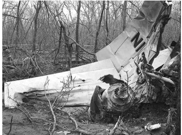
Fig. 34.4. A Cessna 500 Citation crashed in a woodlot shortly after take-off from Wiley Post Airport, Oklahoma City, Oklahoma on 4 March 2008. Analysis of organic remains recovered from the aircraft by a U.S. Department of Agriculture biologist under the direction of the National Transportation Safety Board indicated the aircraft had struck at least one American white pelican ( Pelecanus erythrorhynchos ) during the initial climb (Dove et al. 2009). All 5 people on board were killed. Photo by U.S. Department of Agriculture.
