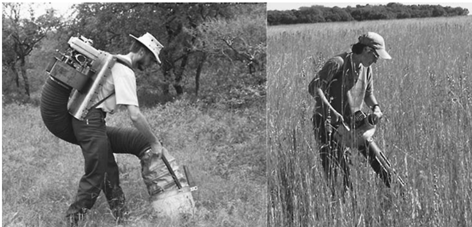
Fig. 14.5. Different types of suction devices. The D-vac (left) is commercially available; the other device is a leafblower (right) with a suction option. Both work well, although the D-vac is more powerful (but less portable). Left photo by L. Sands.
