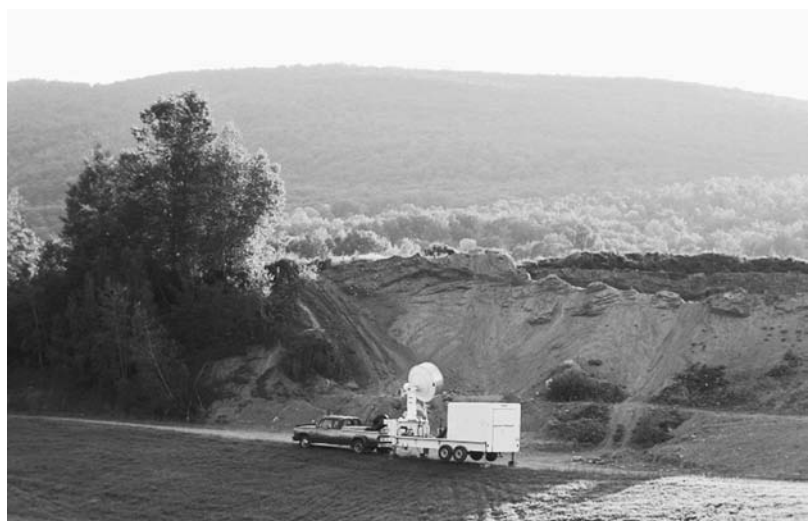
Fig. 13.8. A radar is sited in a gravel pit behind an earth barrier to reduce ground clutter during observations of wildlife flying at low height over a ridge. The operators positioned the trailer-mounted antenna so that the radar’s pencil beam can point low over the ridge in the background, while the earth berm 30 m away shields the radar from side lobe reflections off the ridge itself. The aluminum cuff around the antenna further reduces return from side lobes.
