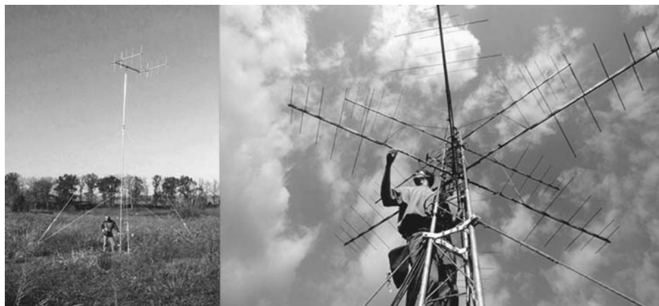
Fig. 10.6. Towers for very high frequency transmitters. System on left has 2–5 element yagi antennas and is collapsible and portable. System on right is a parallel fixed array of log-periodic antennas mounted on a 42.7-m (140 feet) Rohn 25 tower. Photograph on left by J. Millspaugh; photograph on right by R. Kays.
