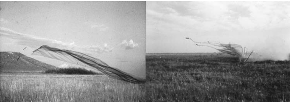
Fig 3.10. Photograph of cannon (left) and rocket nets (right) shortly after being fired. Note how the front end of the rocket net comes off the ground, allowing taller animals to be trapped than could be accomplished with a cannon net. Photo by N.J. Silvy.
