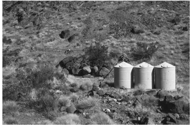
Fig. 27.6. Guzzlers constructed with aboveground storage tanks generally have a float-valve to control the water level in the drinking trough. Guzzlers of this type store up to 10,000 L of water for use by large mammals in the Mojave Desert, California.
