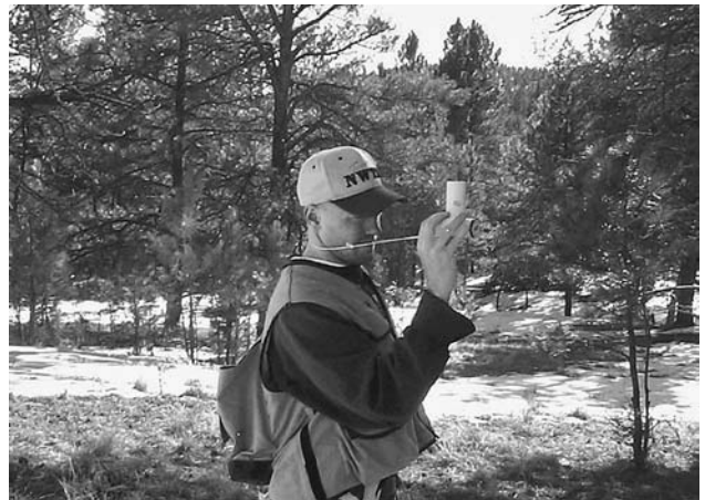
Fig. 16.8. A moosehorn densiometer used to estimate percentage overstory cover in woodlands.
